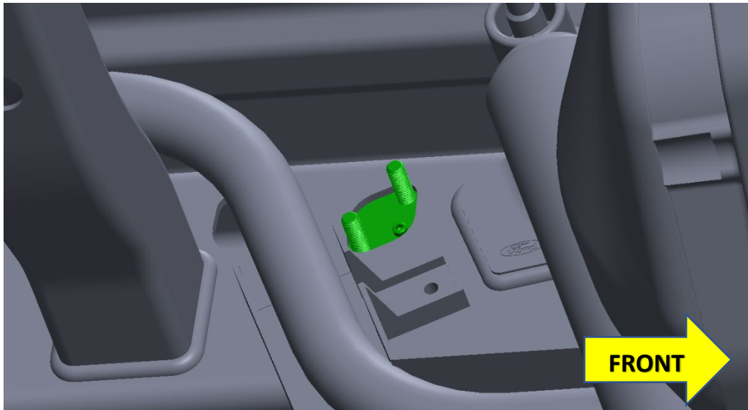
Figure 23- Driver Side Nut Plate Installation
