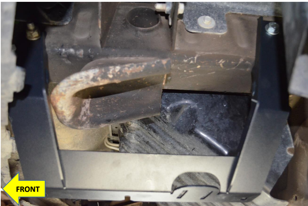
Figure 17 – Bracket Installed to Frame Rail (Shown on Driver Side frame rail with Tow Hook Bolts)
