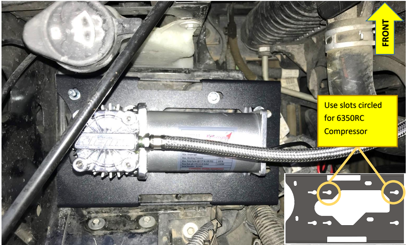
Figure 9 – Compressor Slots and Bracket Orientation Shown (as installed in vehicle)
