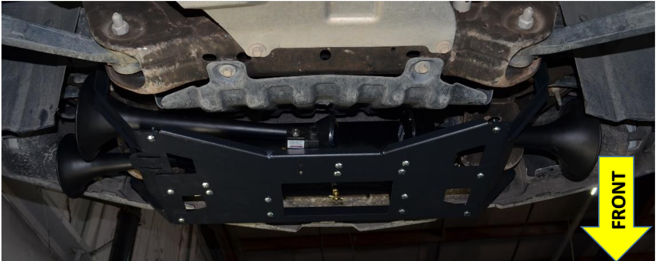
Figure 24 – Trumpets and Kit Installed (as viewed under vehicle looking forward)
