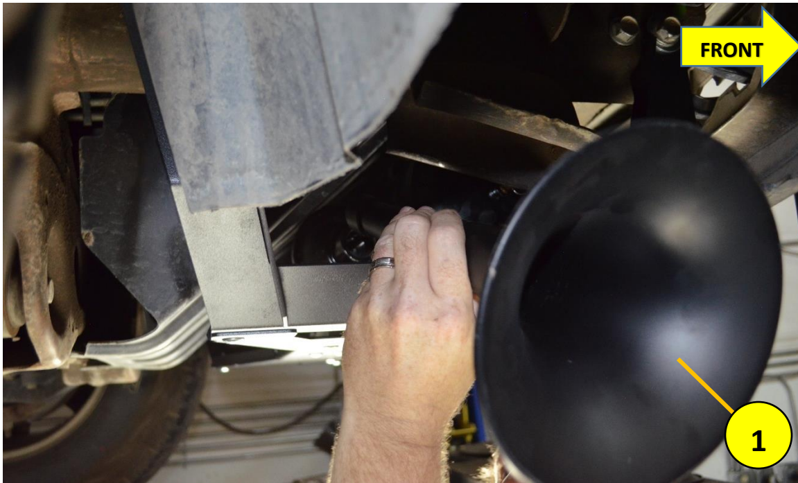
Figure 22 – Installation Orientation of Medium Trumpet (Shown in vehicle on Passenger Side)
