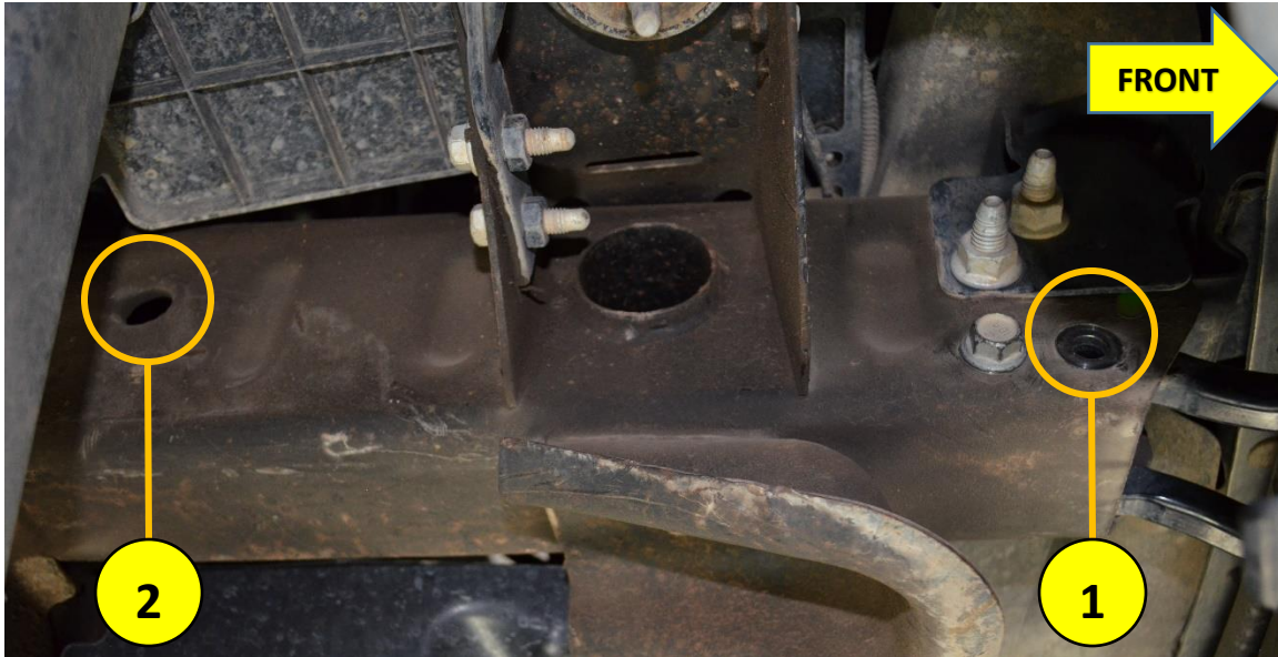
Figure 13 – Frame Attachment Points (Passenger Side of frame shown)
