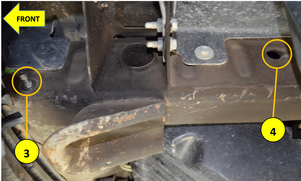
Figure 16 – Frame Rail Attachment Points (Driver Side of frame shown)
