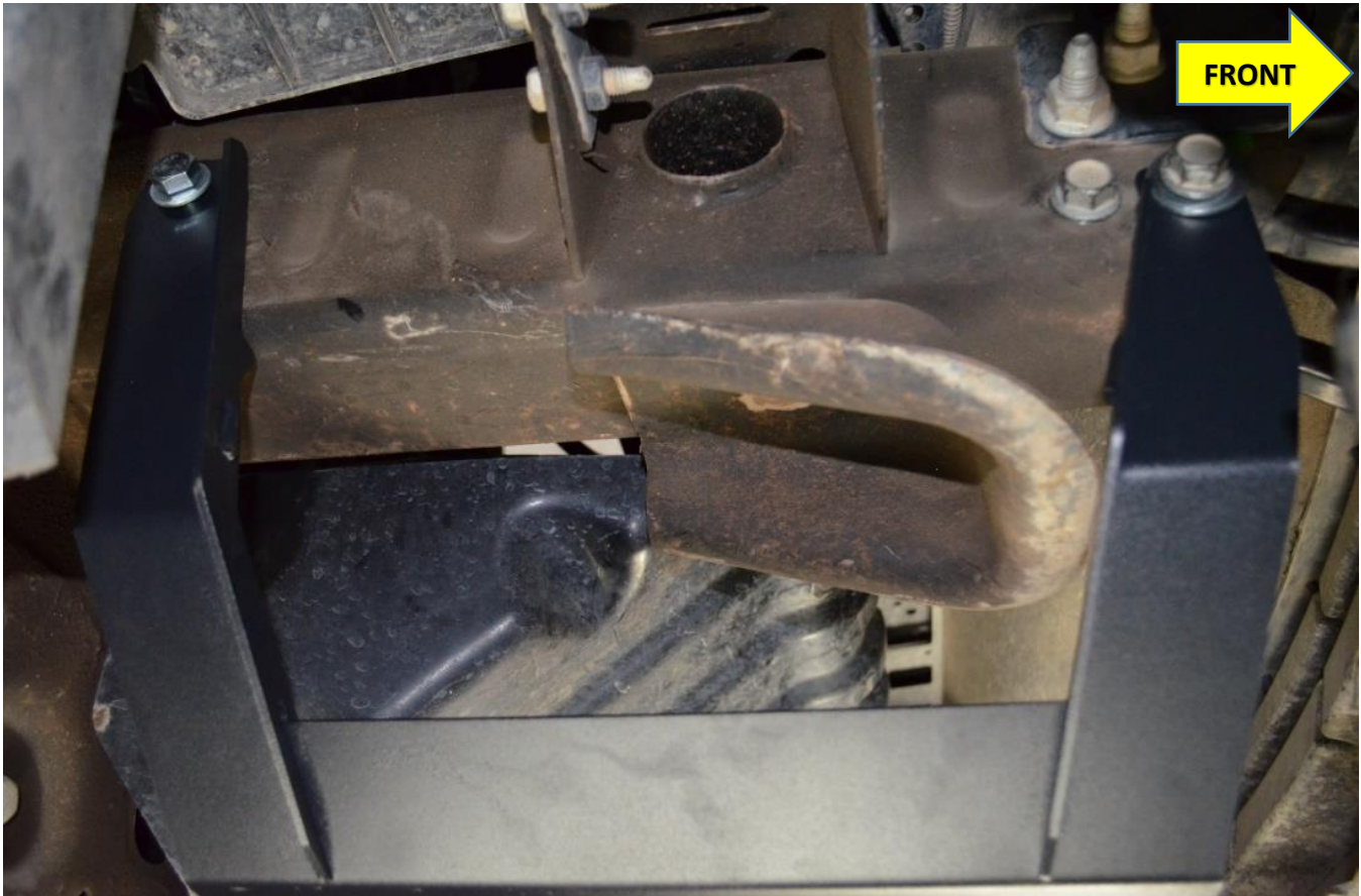
Figure 15 – Bracket Installed to Frame Rail (Shown on Passenger Side frame rail with Tow Hook Bolts)
