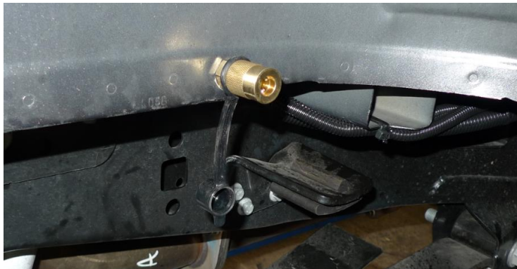
Figure 21 – Example of Quick Connect Coupler Installed inside Rear Fender Well
