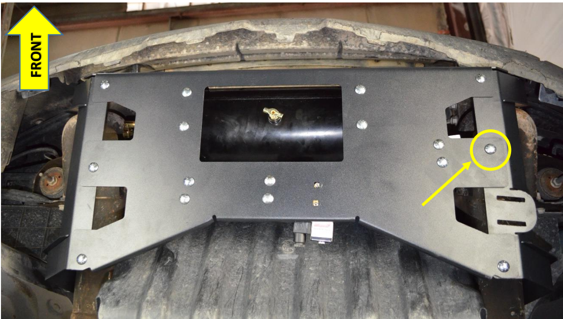
Figure 19 – Air Tank and Air Horn Driver Assembly installed (shown in vehicle)
