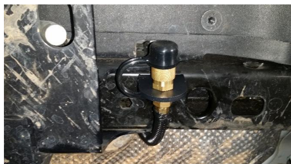
Figure 28 - Example of Air Coupler Mounted below Bumper
