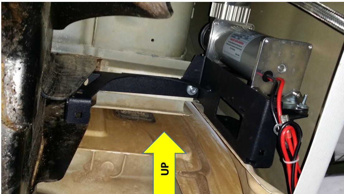
Figure 20 - Air Compressor Bracket Assembly, installed
