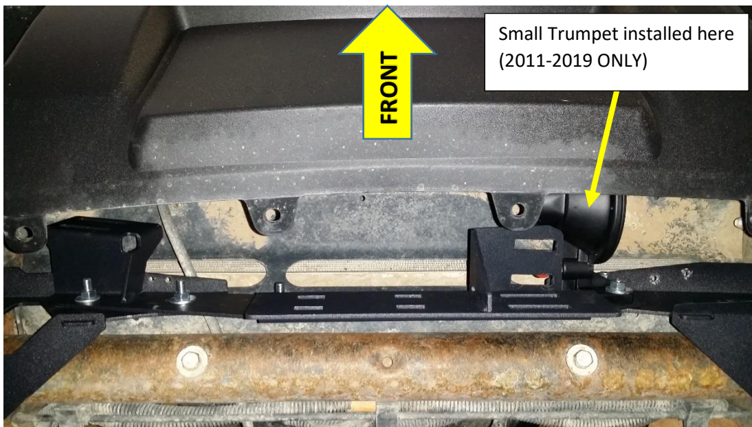
Figure 37 - HD18-303 Connector Bracket, installed (Shown from below)
