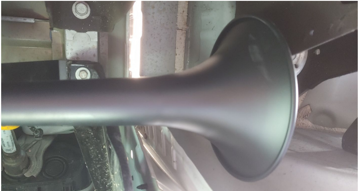
Figure 21- Trumpet Alignment to Prevent Vehicle Contact
