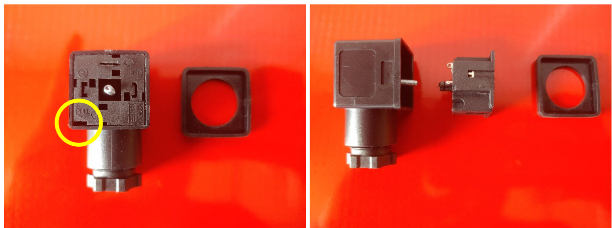
Figure 50- Connector / Housing Separation
