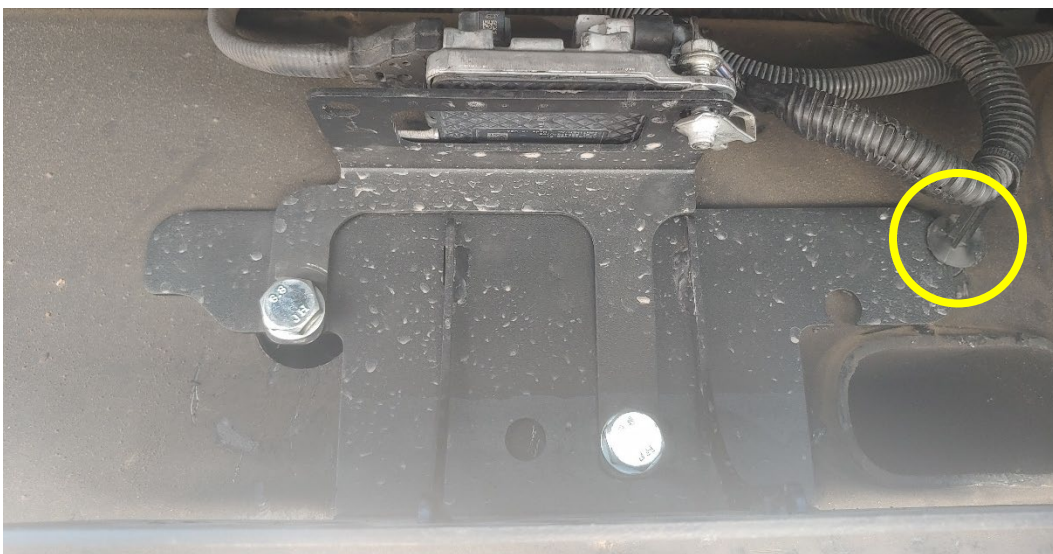
Figure 40- Compressor Bracket Installation 2, Diesel
