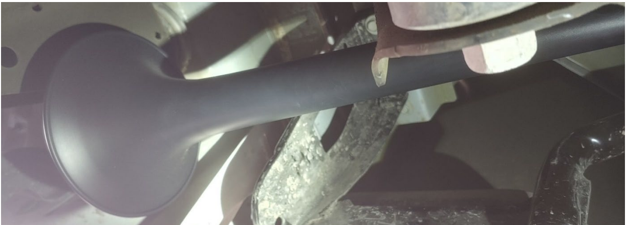
Figure 26- Trumpet Alignment to Prevent Vehicle Contact
