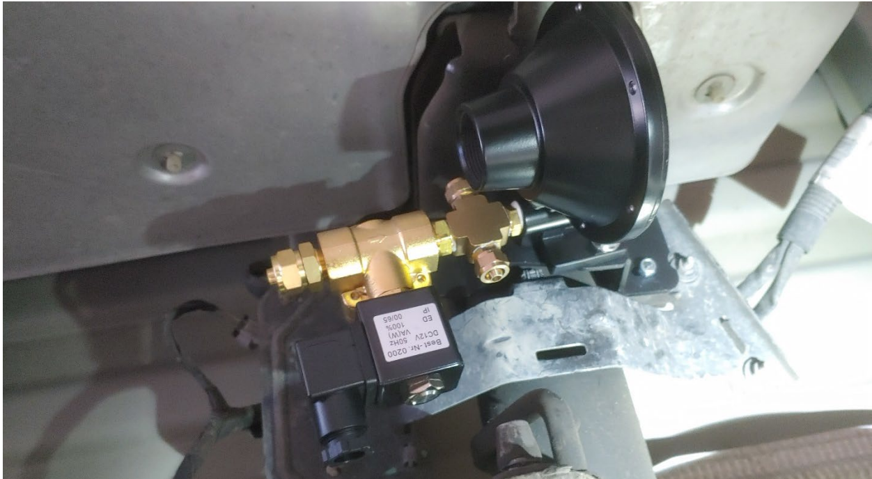
Figure 30- Center Air Horn Bracket & Driver Temporarily Attached ( Shown Without Air Tubing for Clarity )
