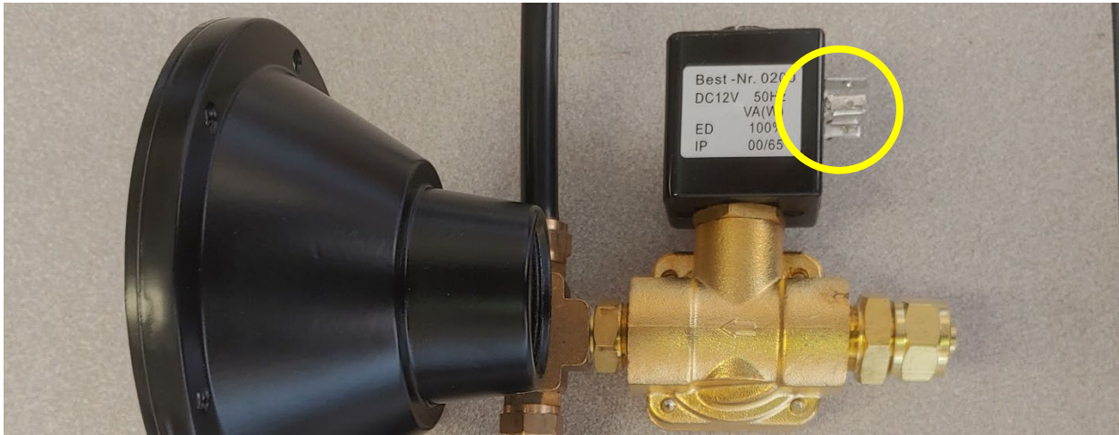
Figure 10- Solenoid Electrical Connector Removal
