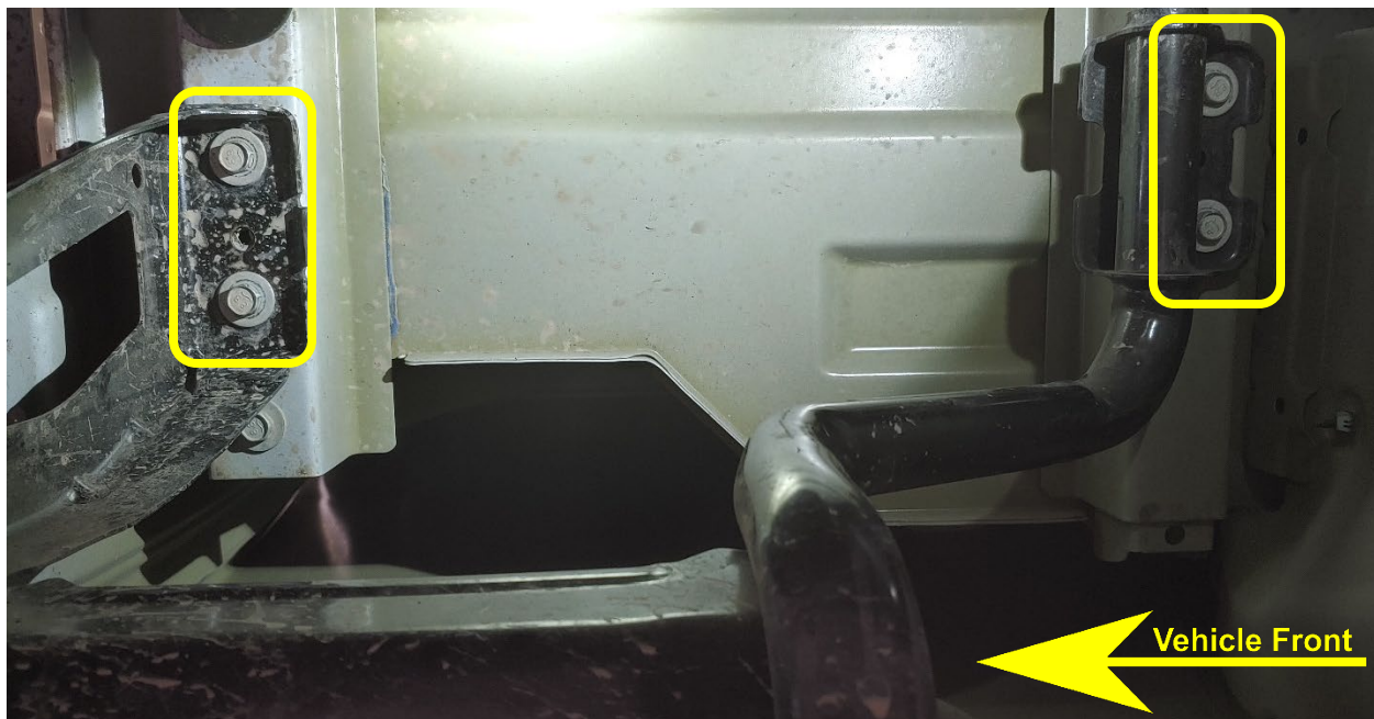
Figure 24- Passenger Side Horn Bracket, Mounting Points
