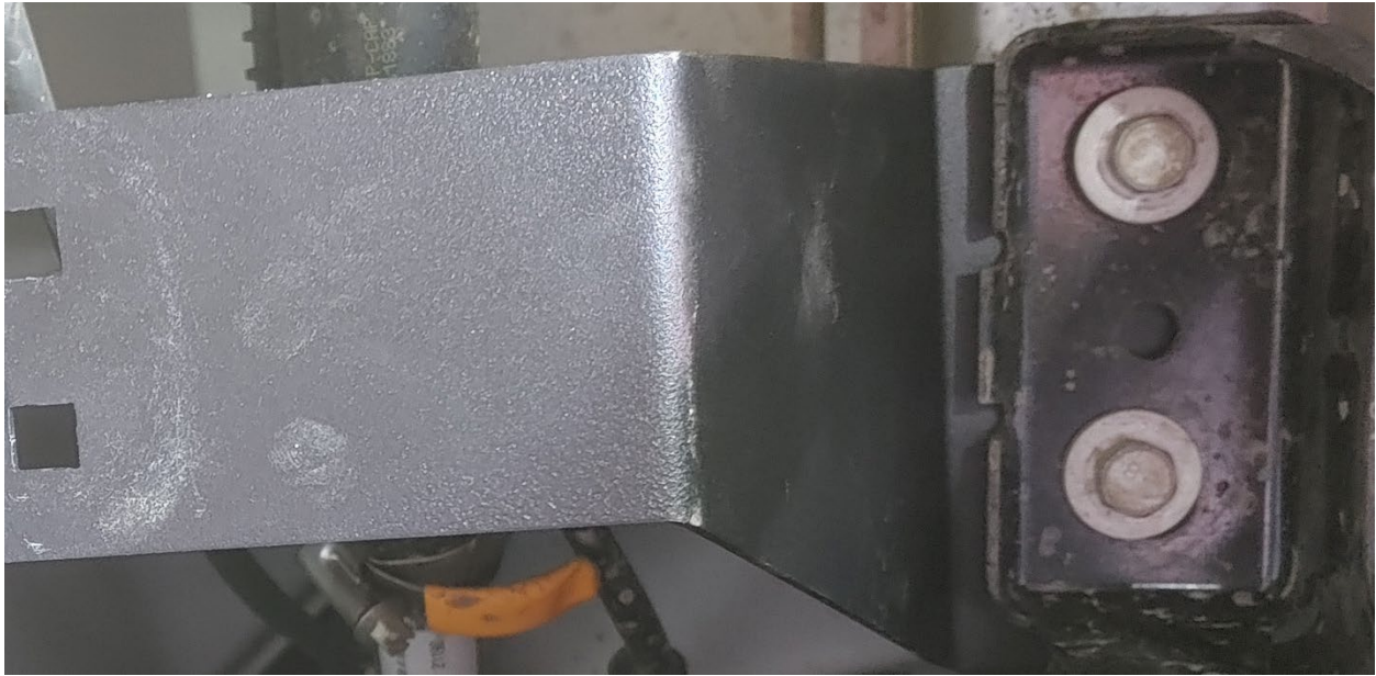
Figure 18- Driver Side Bracket Install, Frontmost Location
