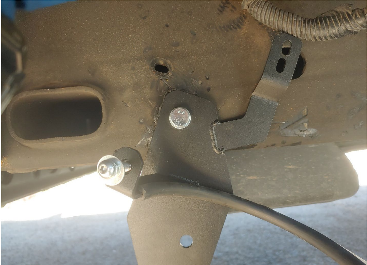
Figure 45- Tank Bracket Installation 1, Diesel
