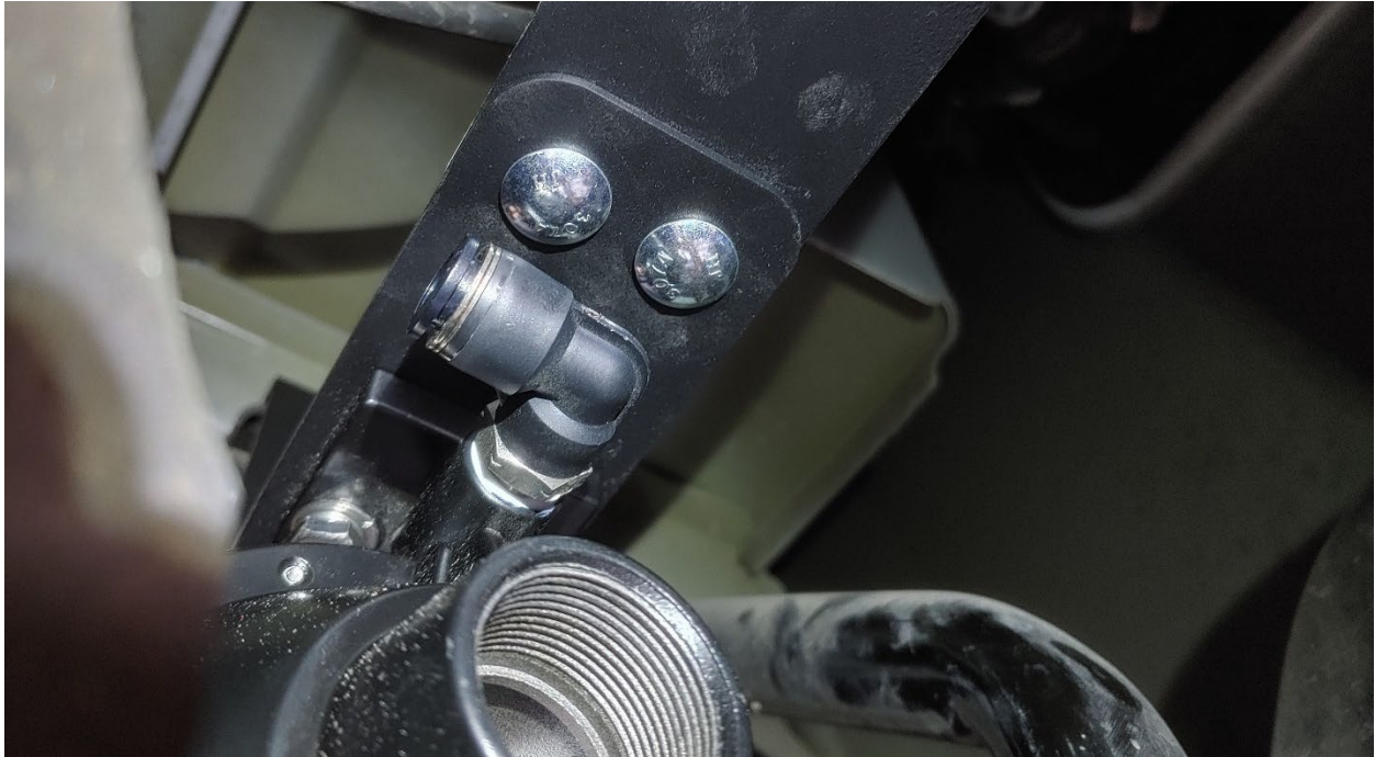
Figure 20- Driver Side Bracket Install, Brackets Temporarily Secured
