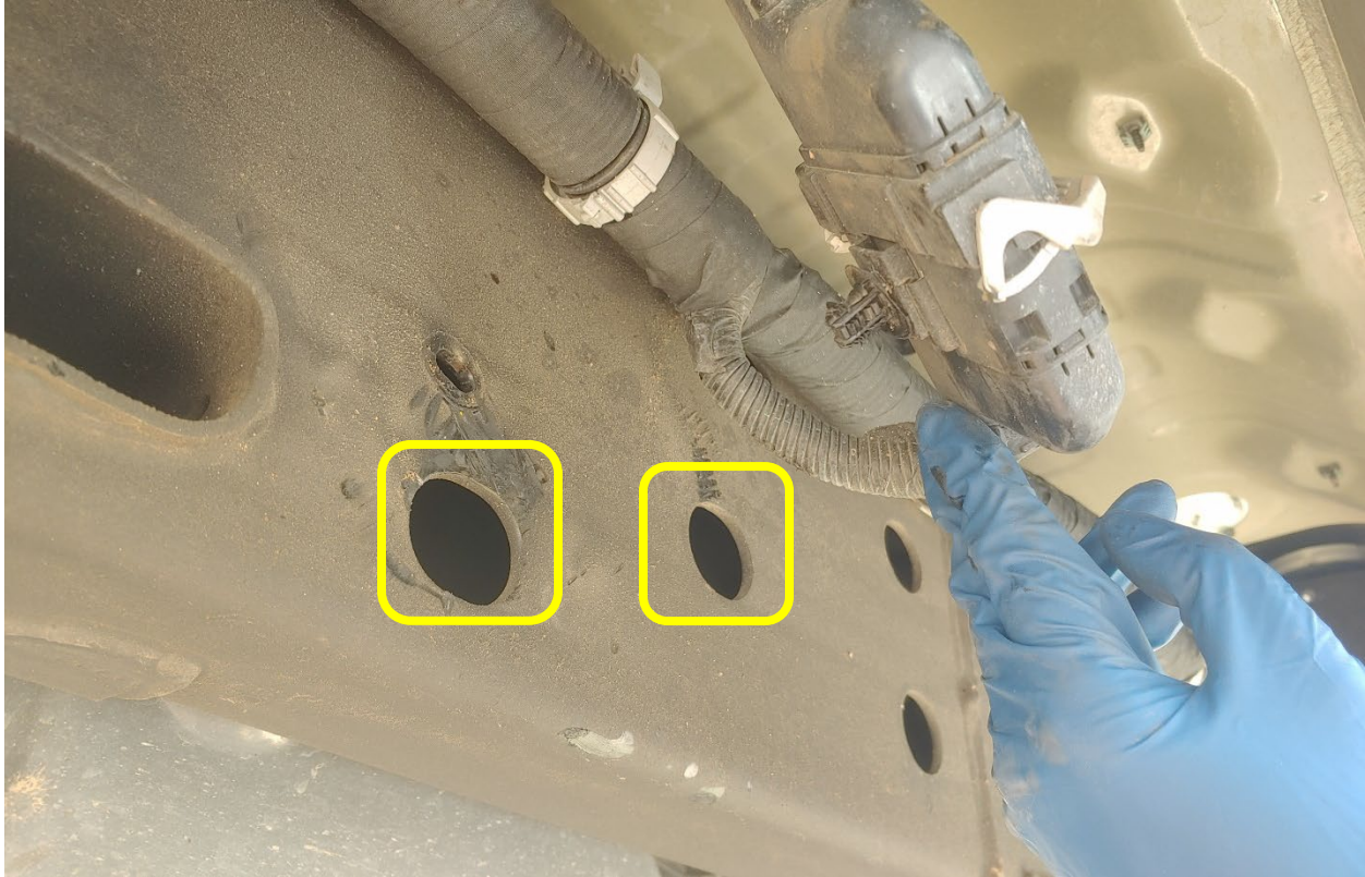
Figure 42- Tank Frontmost Bracket, Mounting Point
