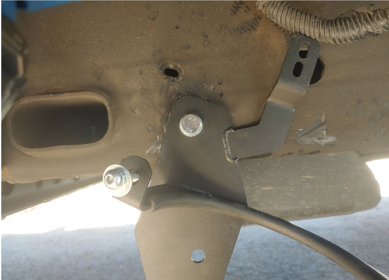
Figure 21- Tank Bracket Installation 1, Diesel
