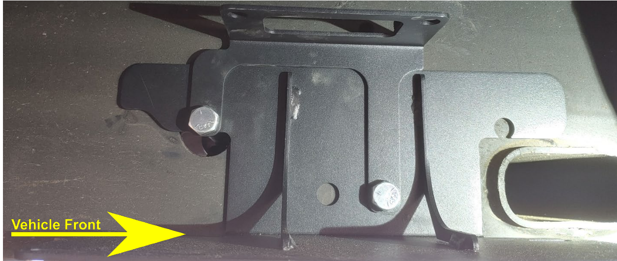
Figure 11- Compressor Bracket Installation, Outside Frame Rail
