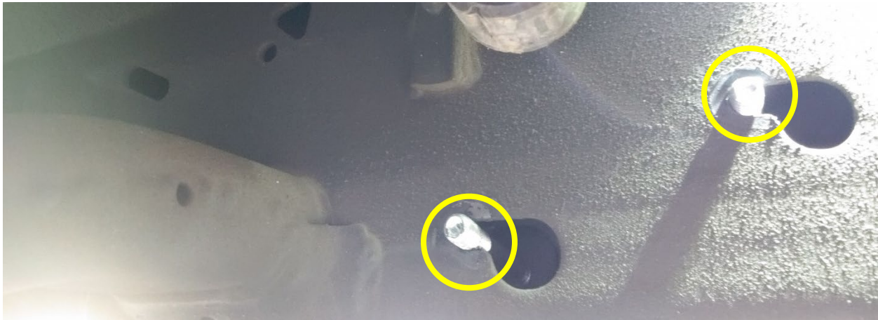
Figure 19- Tank Bracket Installation, Inside Frame Rail
