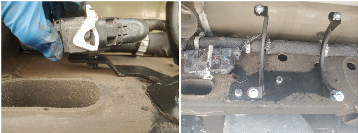
Figure 20- Tank Bracket Installation, Connector Placement
