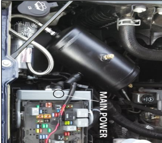
Figure 11: Air Compressor & Tank Install (A & C)
