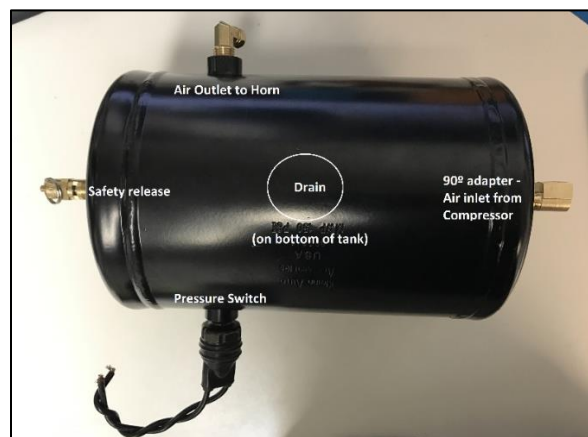
Figure 7: Air Tank Fittings (B & D)
