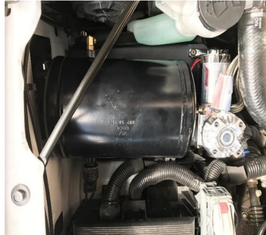
Figure 12: Air Compressor & Tank Install (B & D)
