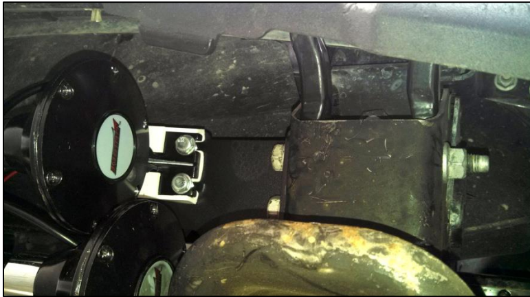
Figure 5: Horn Mount Installed with Tow Hook:
