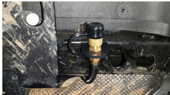
Figure 37 – Example of Air Coupler Mounted to Bumper
