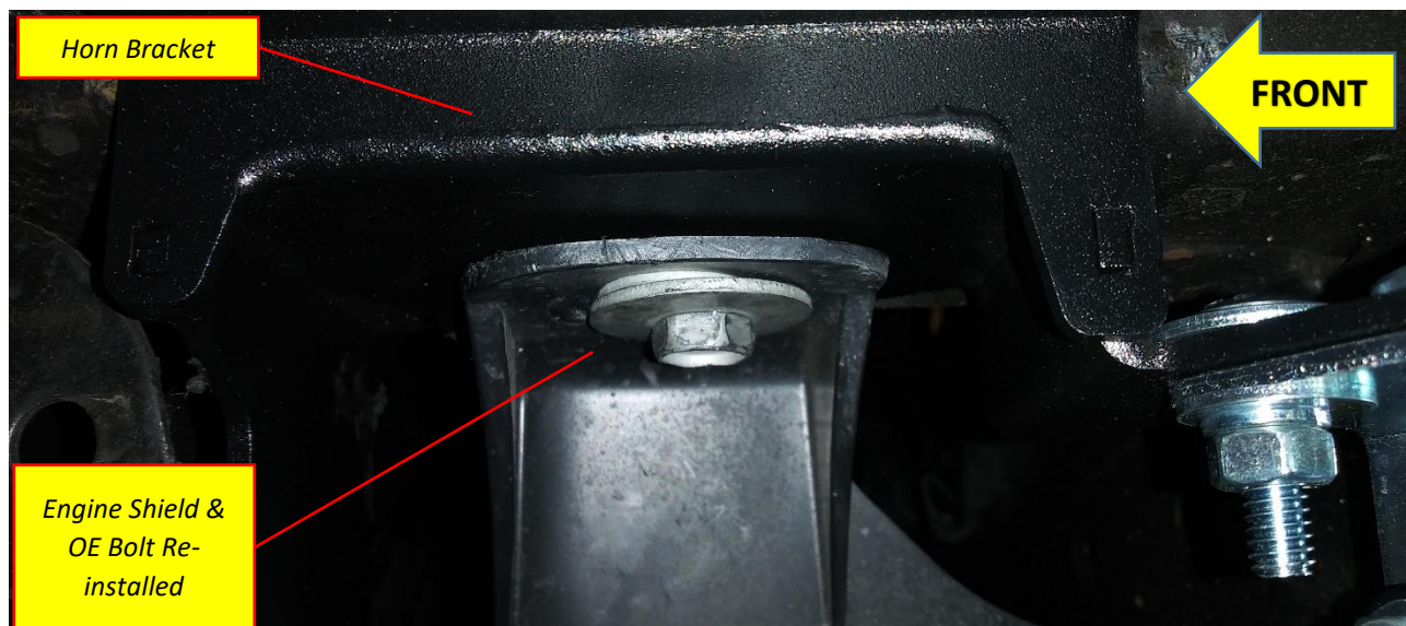
Figure 29 – Air Horn Sub-Assembly installed with Engine Shield in place (2020 Silverado Shown)
