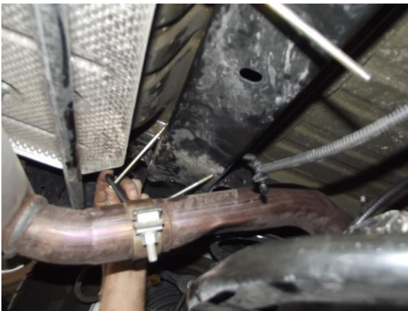
Photo 3 – Slide the rear mount plate/bolt assemblies over the beam. Work from the driver’s side and slide the assemblies towards the passenger’s side
