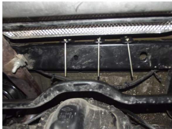
Photo 4 – All three rear mount plate/bolt assemblies in place.
