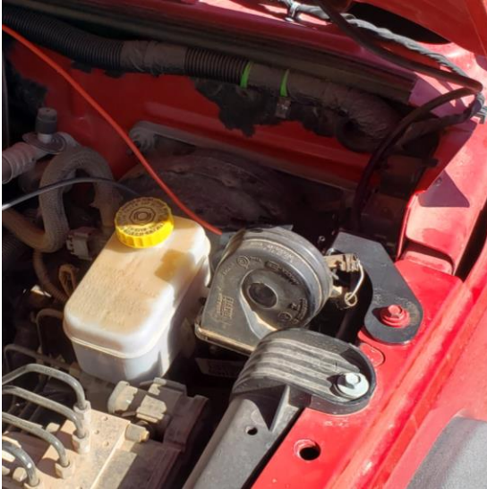
Figure 11: HydroBlast Installed (2015 JK Shown)
