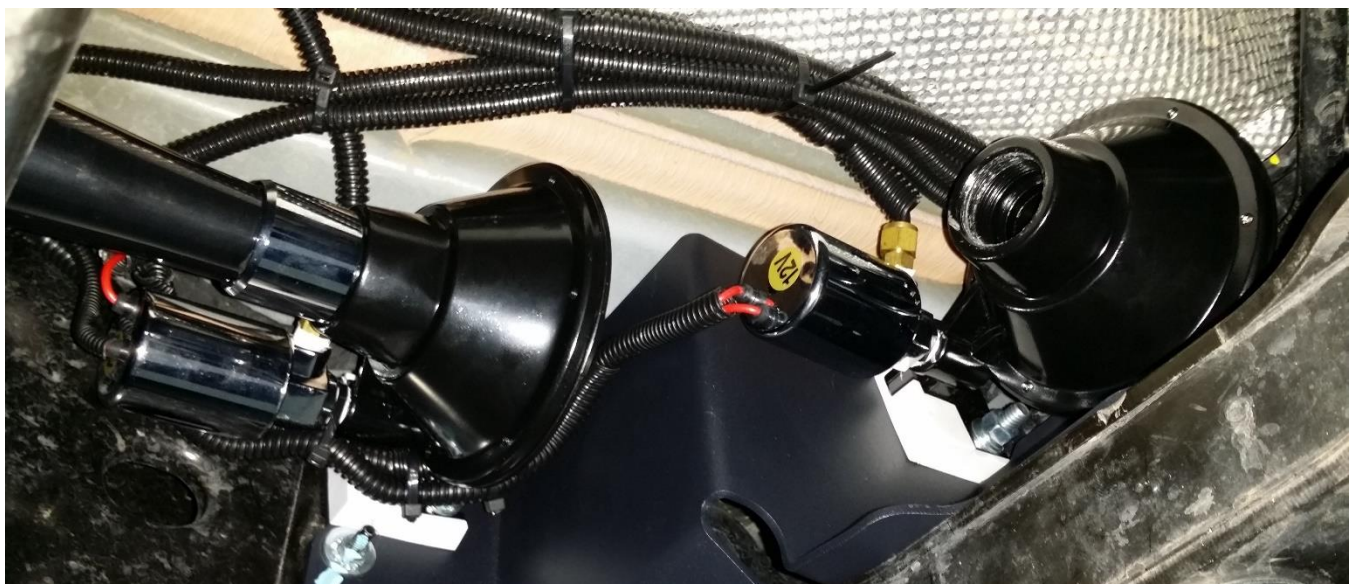
Figure 11 - Horn Assembly Installed w/ Wiring and Air Lines
