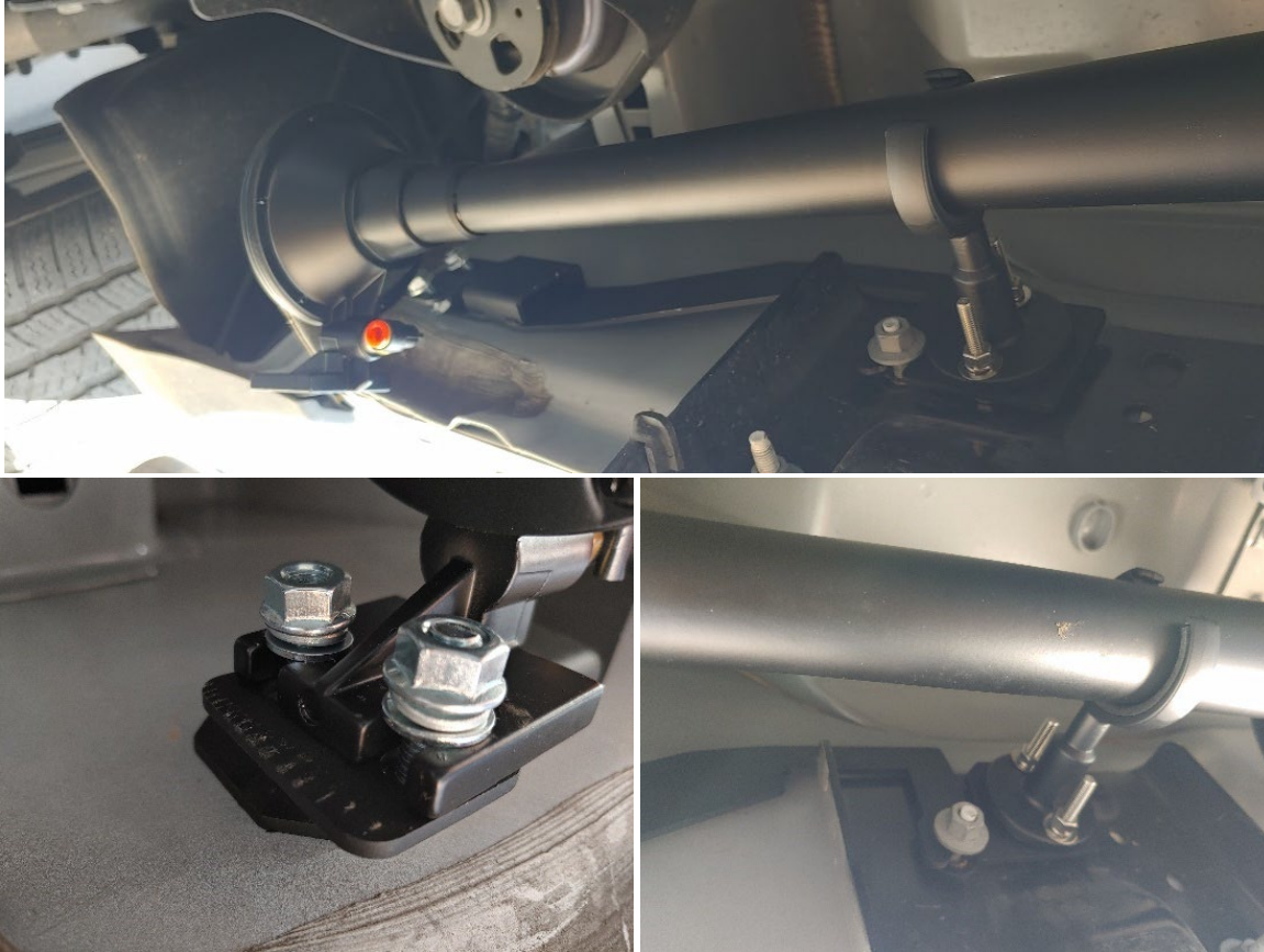
Figure 23- Large Horn Installation
