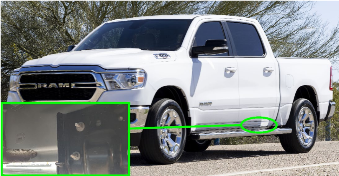
Figure 21- Large Horn & Horn / Ore Bracket Location
