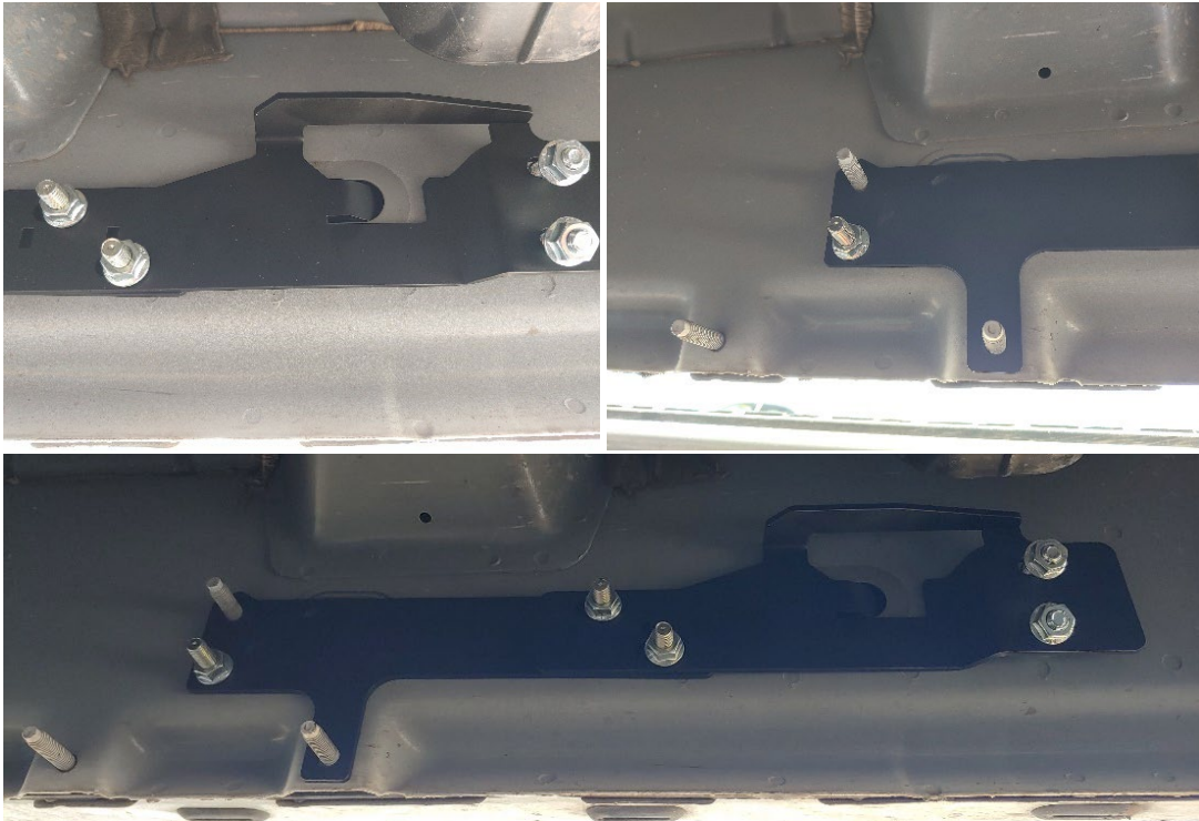
Figure 26- Dual Horn Bracket Installation 1
