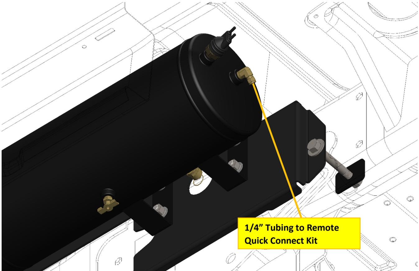
5. Connect remote air compressor filter kit (included with compressor) and route, as desired
