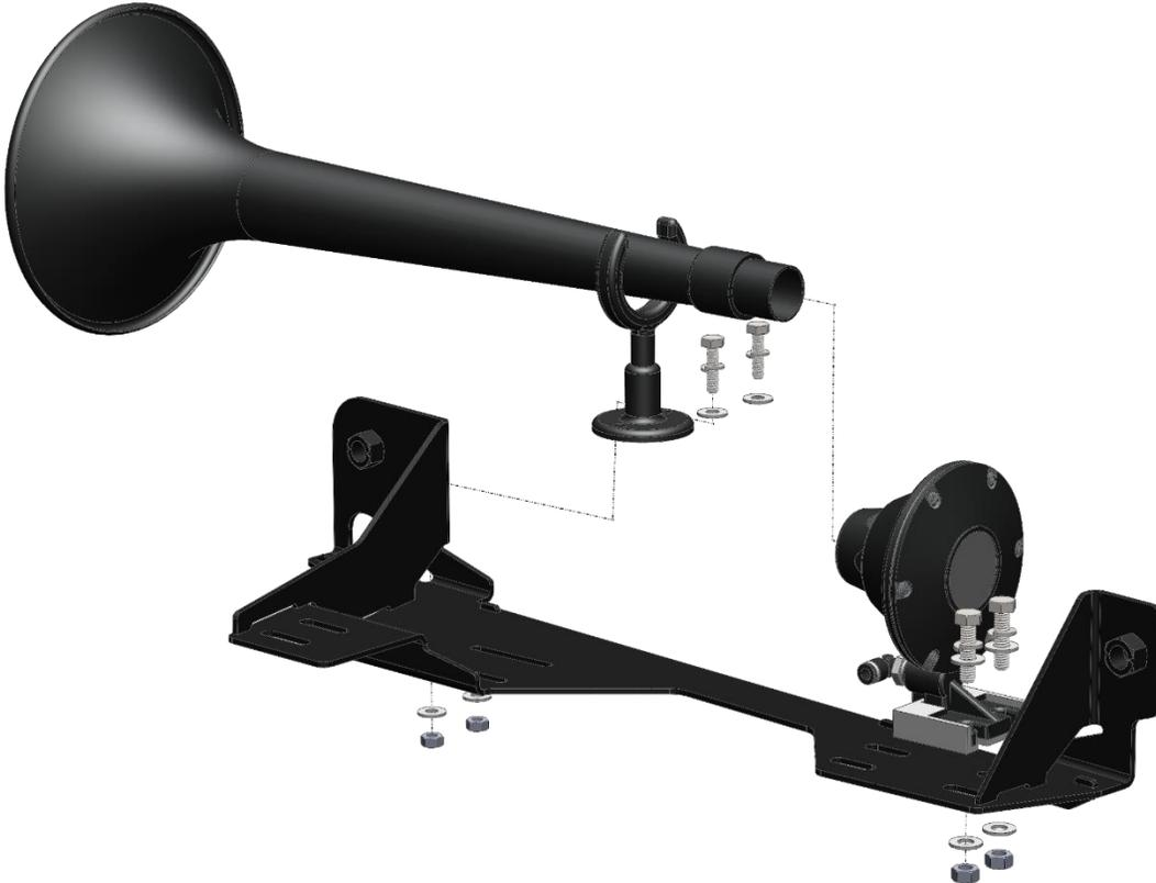
2. Attach Air Solenoid and fitting to Horn Driver with built-in tee and attach to bracket, per below illustration.
