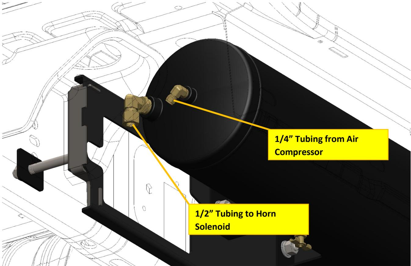
3. Connect Medium Air Horn solenoid to air tank outlet using supplied 1/2" tubing
