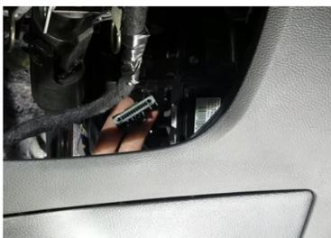
① Gateway module, located at right of steering column, Back view, 24-pin black connector.
