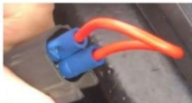
**STEP 3:** Connect the remote start harness to the Gateway Plug
