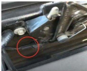
Take the Red wire from the Accessory Pack to use as a jumper to connect the two pins in the hood pin plug as shown below.
