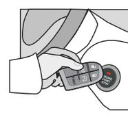
Place the OEM remote (no battery) close to the front of START/STOP button as shown.
