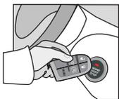
Place the OEM remote (no battery) close to the front of START/STOP button exactly as shown. Do not move the OEM remote for the following step.
