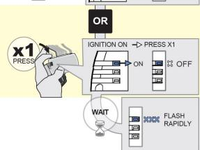
If the LED remains lit solid BLUE after the ignition is turned on, then press and release the programming button once (1x).
