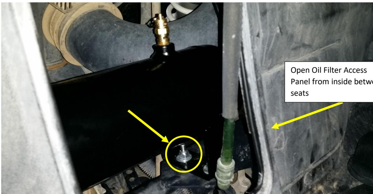
Figure 25 - Access to Air Tank Feet Bolts through Firewall
