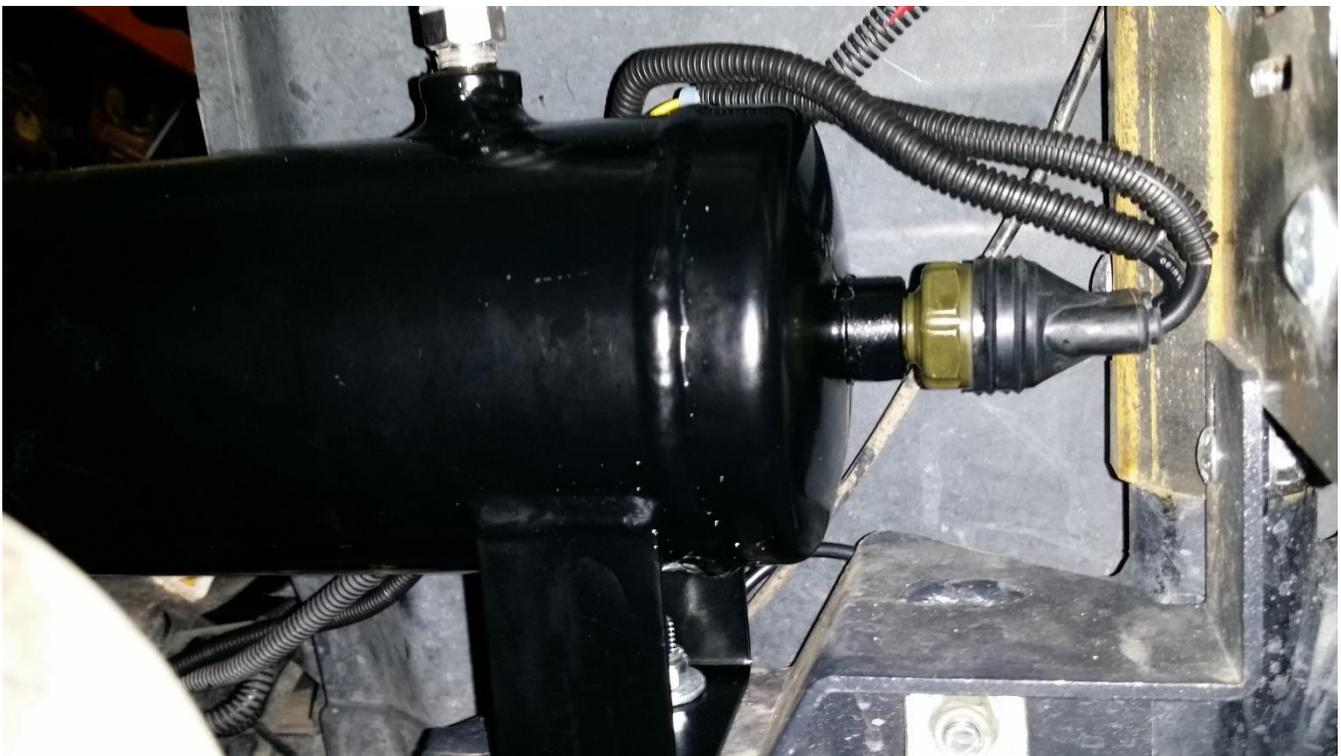
Figure 22 - Air Tank Installed with Pressure Switch Wired
