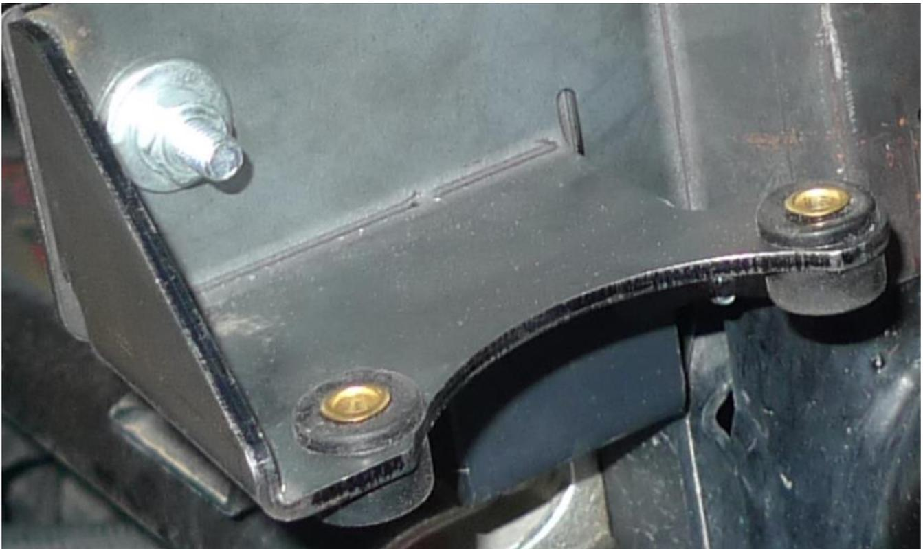
Figure 8 - Air Compressor Bracket with Rubber Grommets Installed
