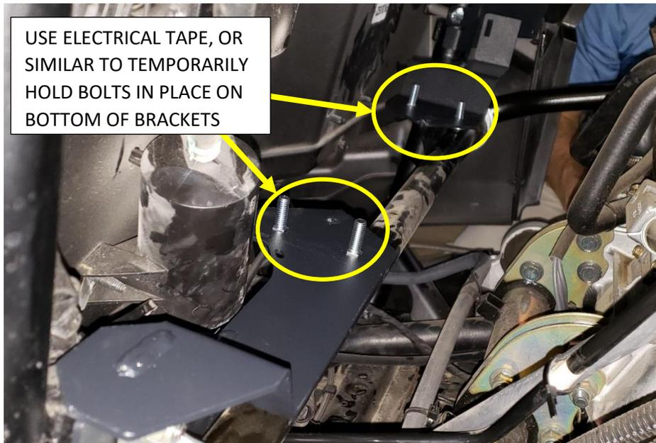
Figure 14 - Air Tank Brackets with Air Tank Bolts taped to bottom
