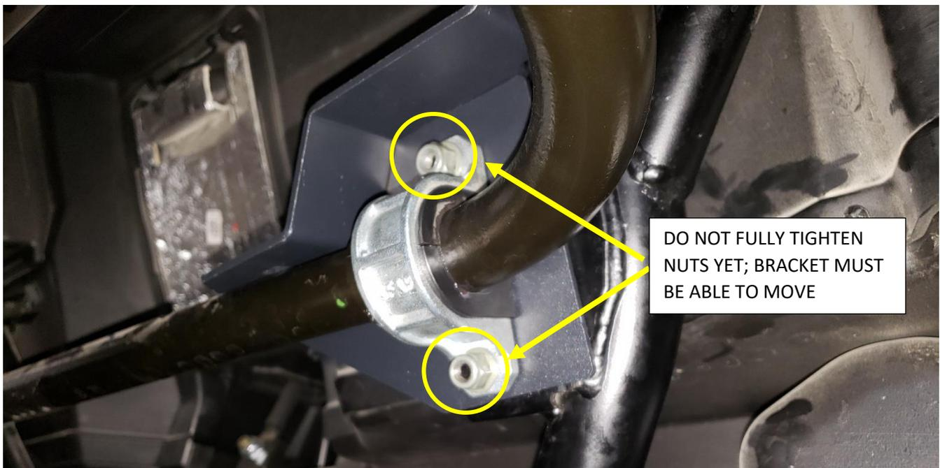
Figure 17 - Driver Side Sway Bar Nuts/Bolts with Air Tank Bracket Inserted
