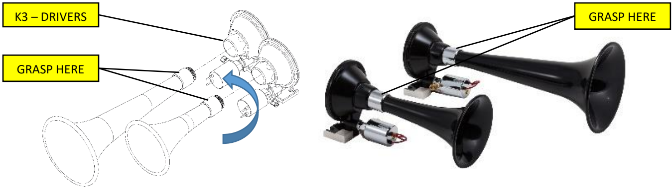
Figure 7 – Removing Trumpets from Air Horn Drivers, Exploded View
