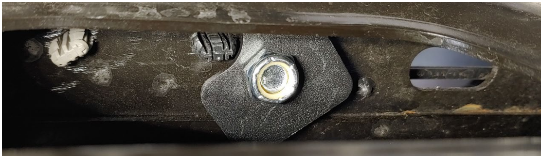
Figure 20- Cutaway Washer Secured via Nylon Lock Nut
