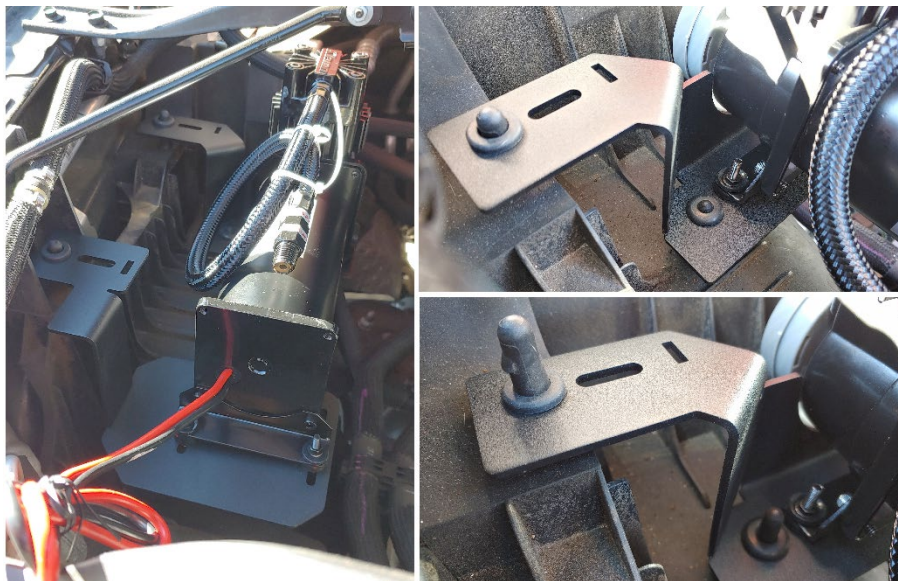
Figure 12- Compressor Bracket, Installed
