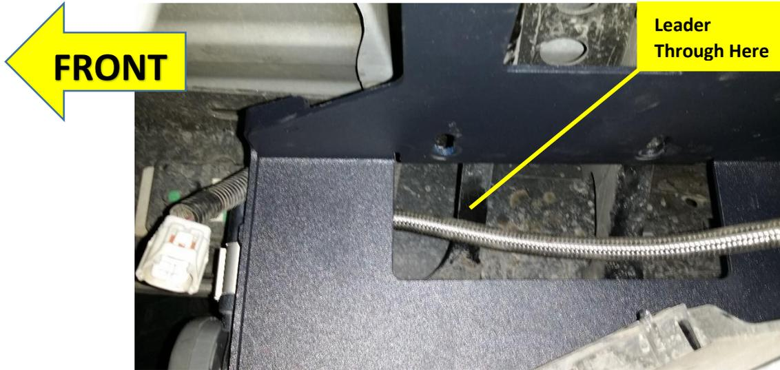
Figure 10 - Compressor Leader Hose Routing
