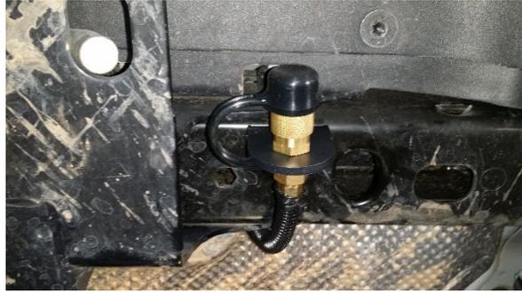
Figure 20 – Example of Air Coupler Mounted To Bumper
