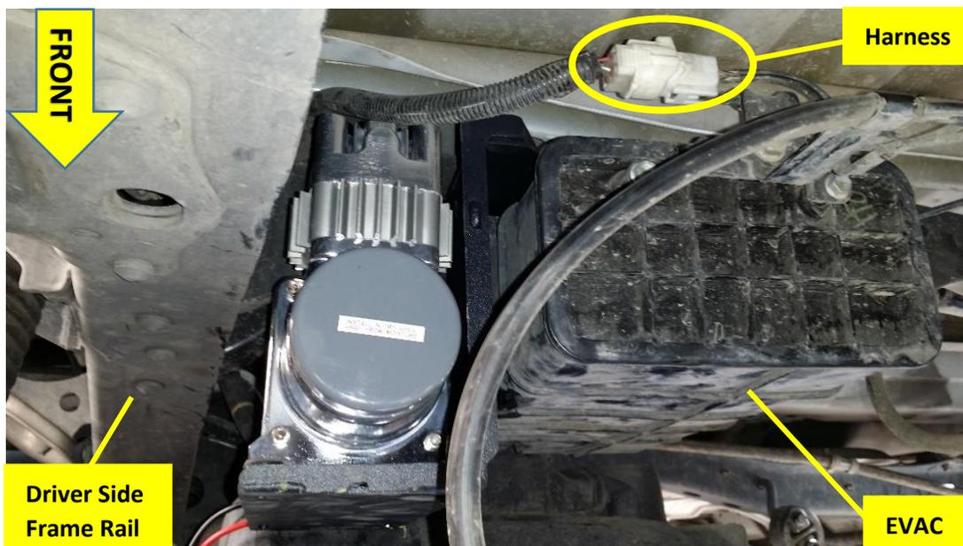
Figure 9 - TUNDRA-301 and Air Compressor Mounted next to EVAC
