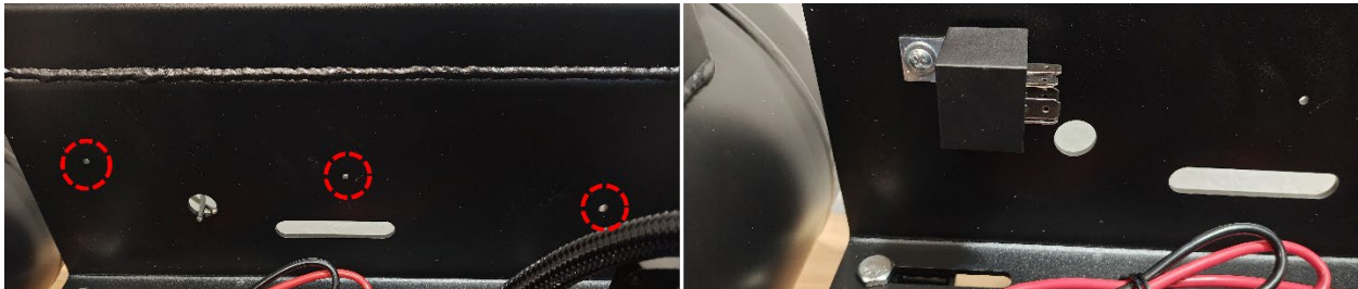
Figure 17- Relay Installation - USTL Bracket Option
