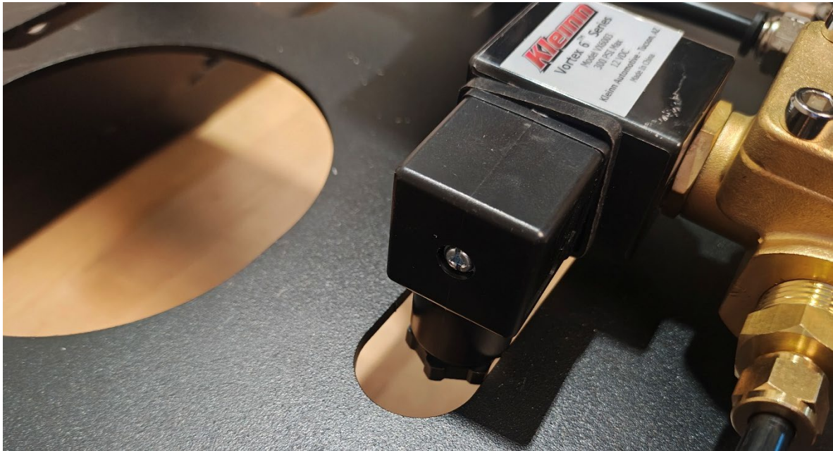
Figure 14- Electrical Connection Reconfiguration
