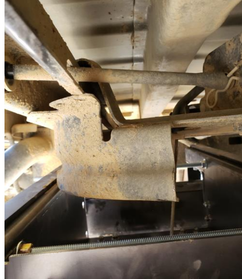
Figure 2: RAM Spare Tire Location Fitment
