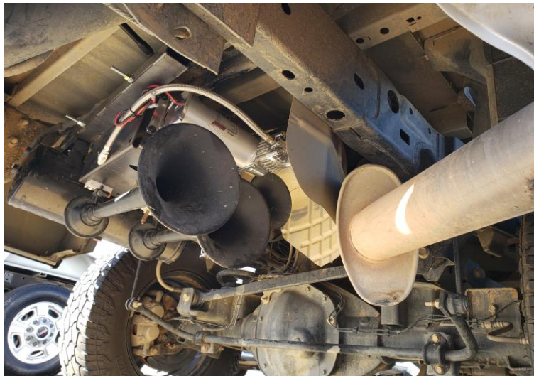
Figure 3: RAM Trumpets Passenger Side Installation
