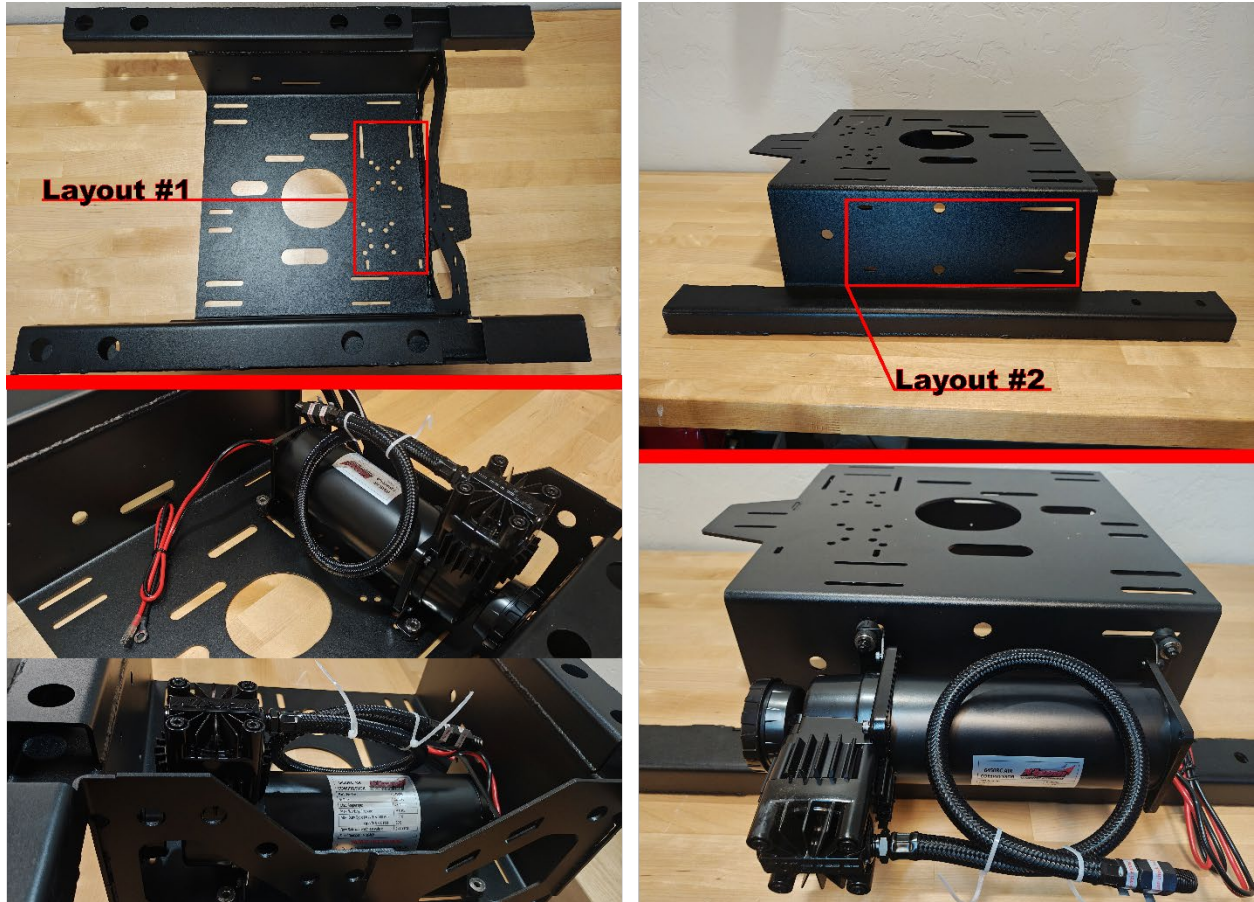
Figure 3- Compressor Installed. Layout 1 (left) & Layout 2 (right)
