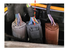
Junction Module connector Behind Glove Box
