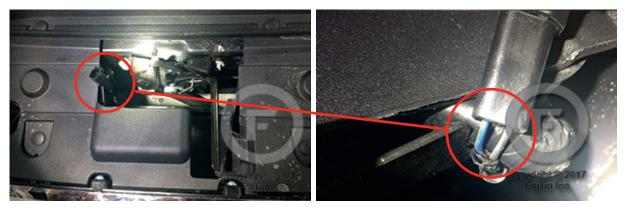
STEP 3: Connect the remote start harness to the Gateway Plug
