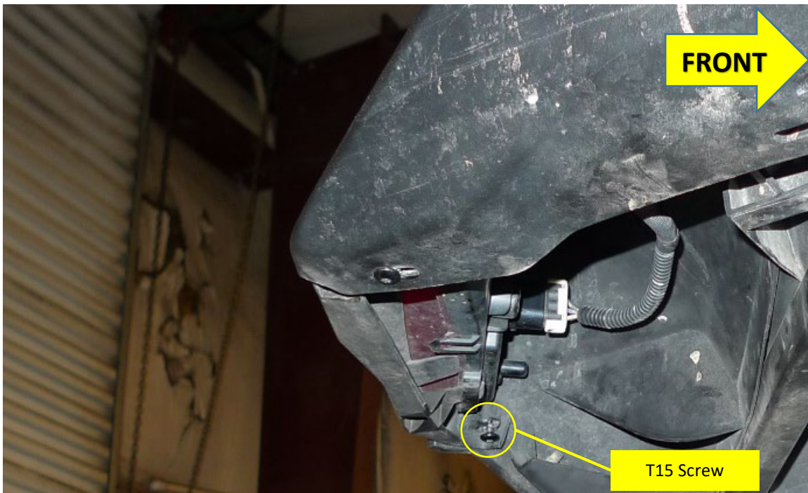
Figure 4 – Passenger Rear Fender Removal (below taillight)
