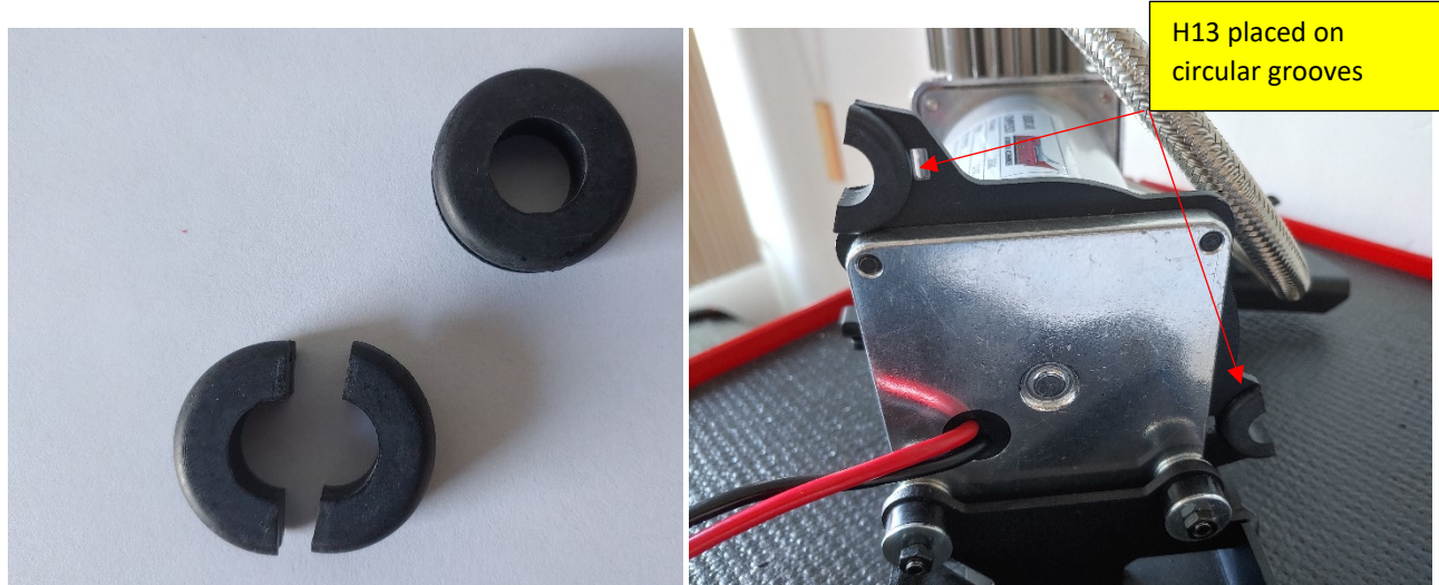
Figure 17- H13 Cut & Installed
