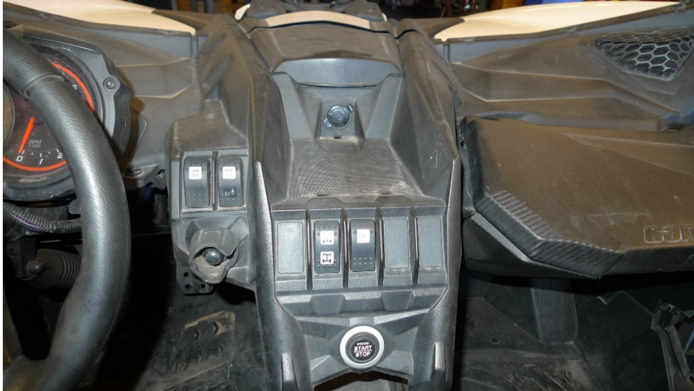
Figure 41- Center Console for Rocker Switch Install
