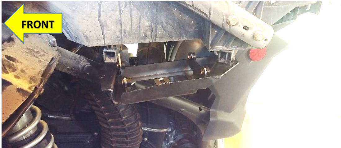
Figure 25 – Air Compressor Bracket Final Install (Shown installed on CARB Vehicle)
