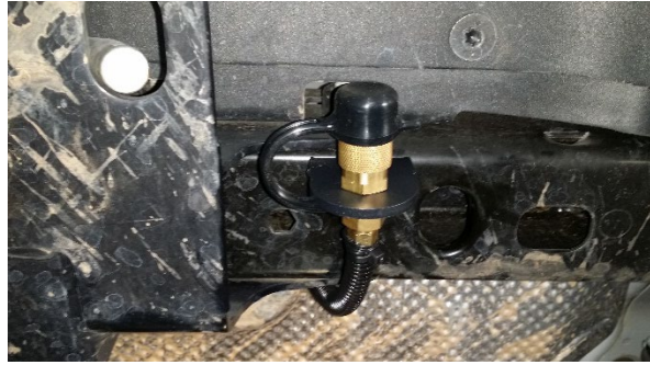
Figure 38 – Example of Air Coupler Mounted to Bumper
