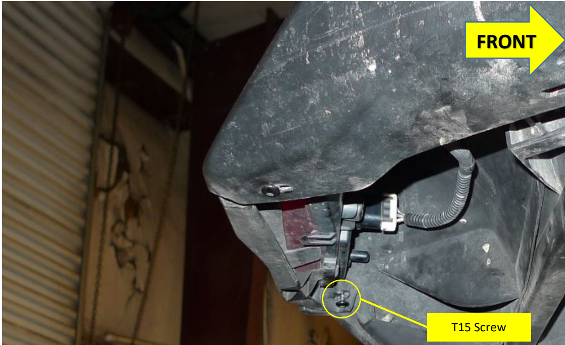
Figure 4 – Passenger Rear Fender Removal (below taillight)
