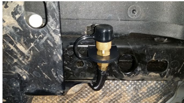
Figure 29 – Example of Air Coupler Mounted to Bumper
