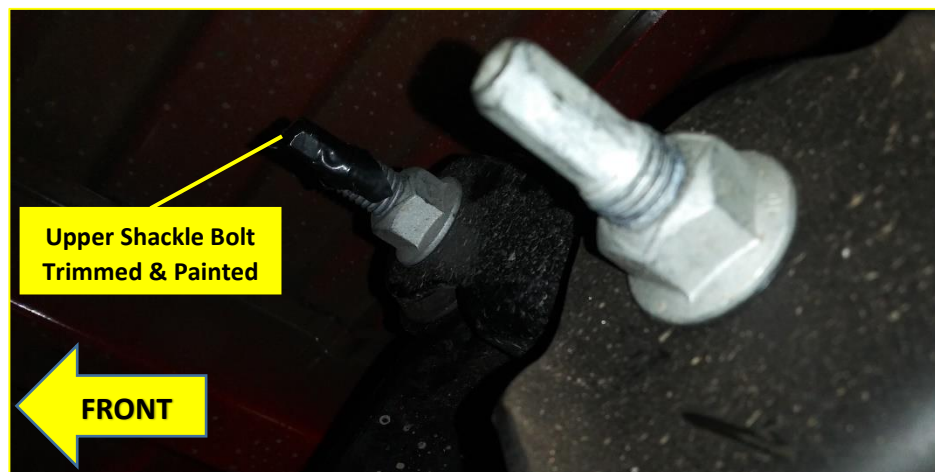
Figure 16 – Underbody view of Driver's side Leaf Spring Shackle Bolt trimmed (2020 Silverado shown)
