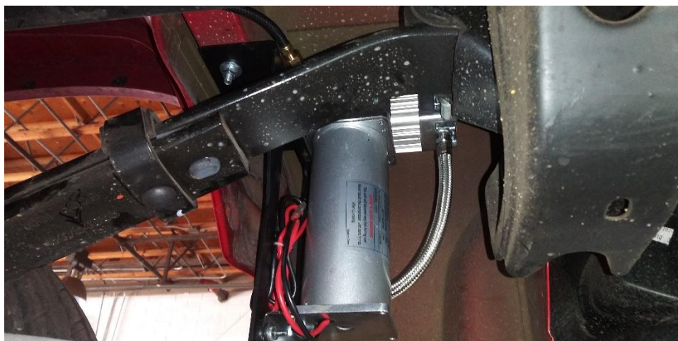
Figure 4 – Under Vehicle view of Air Compressor Installed – Behind Passenger Wheel (2020 Silverado Shown)
