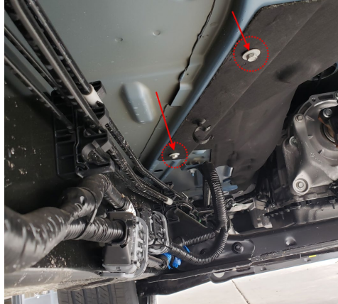
Figure 16- Horn Bracket Install Location
