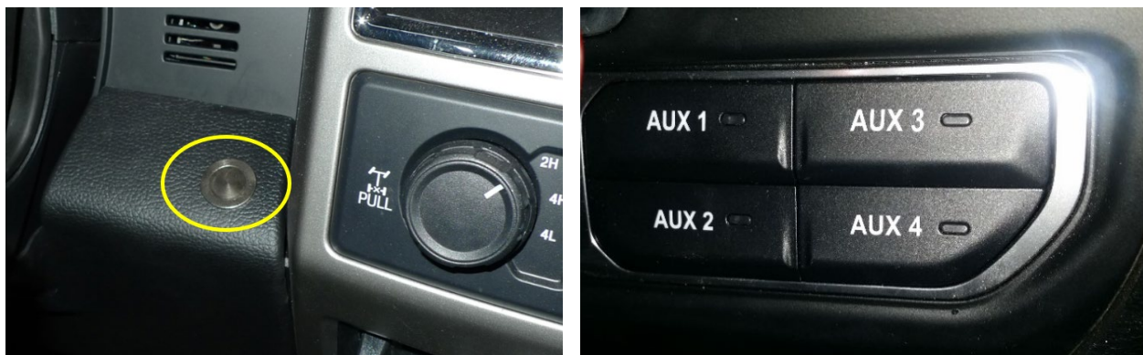
Figure 22: Horn Button Installed / OEM Upfitter Switches
