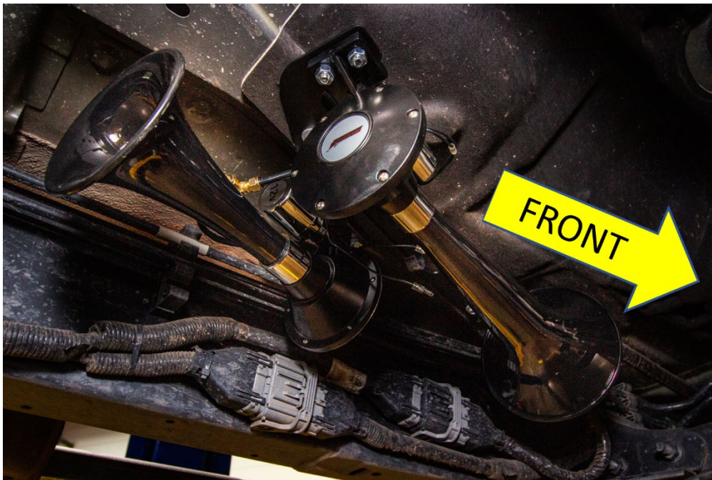
Figure 3: Under Vehicle View (Horns) – Under Driver Side Seating Area (220 Horns Shown)
