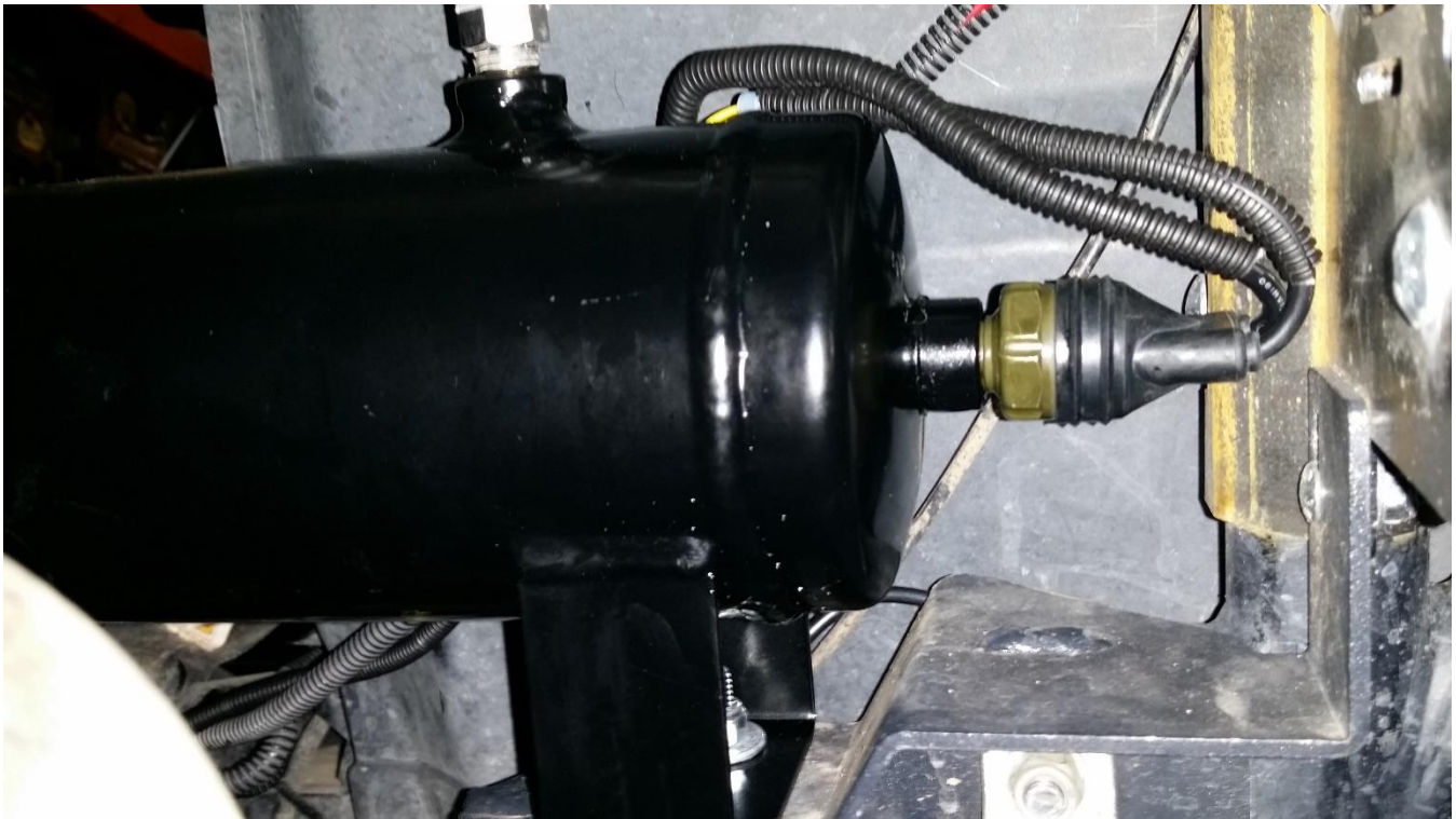
Figure 19 - Air Tank Installed with Pressure Switch Wired
