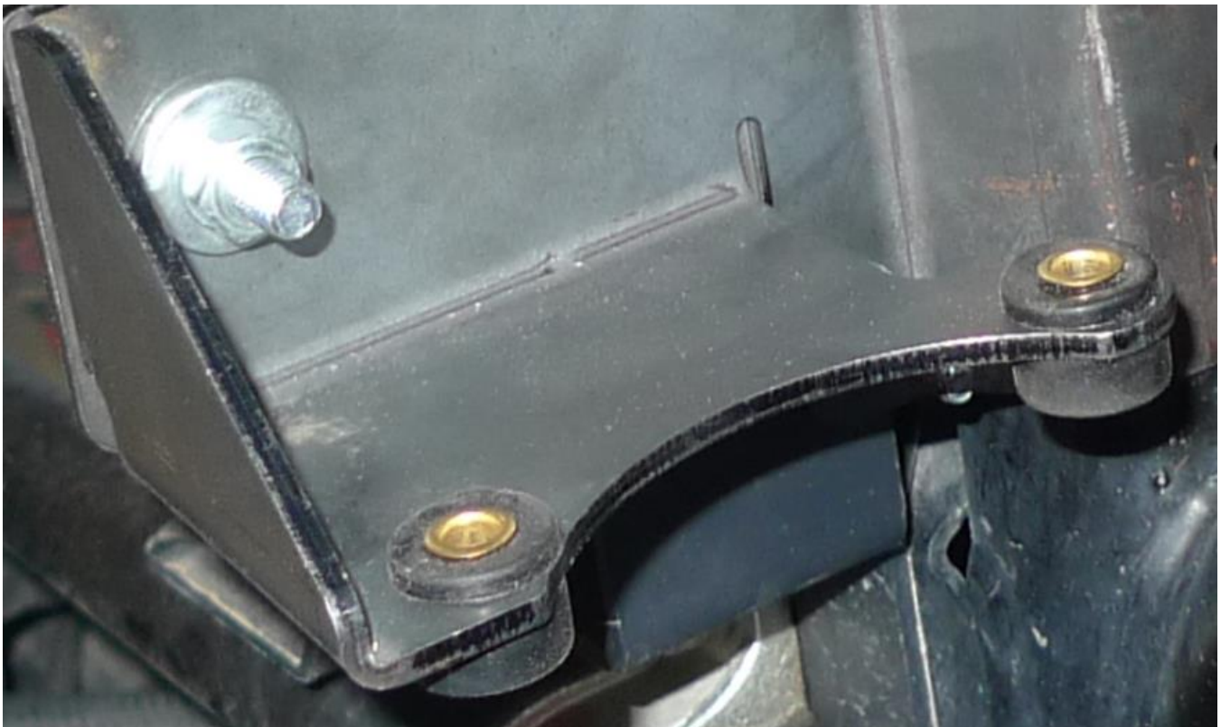
Figure 7 - Air Compressor Bracket with Rubber Grommets Installed
