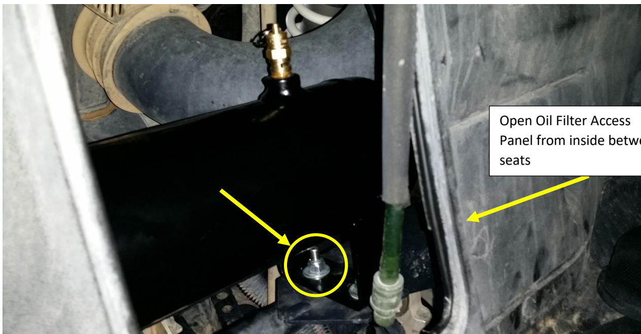
Figure 22 - Access to Air Tank Feet Bolts through Firewall
