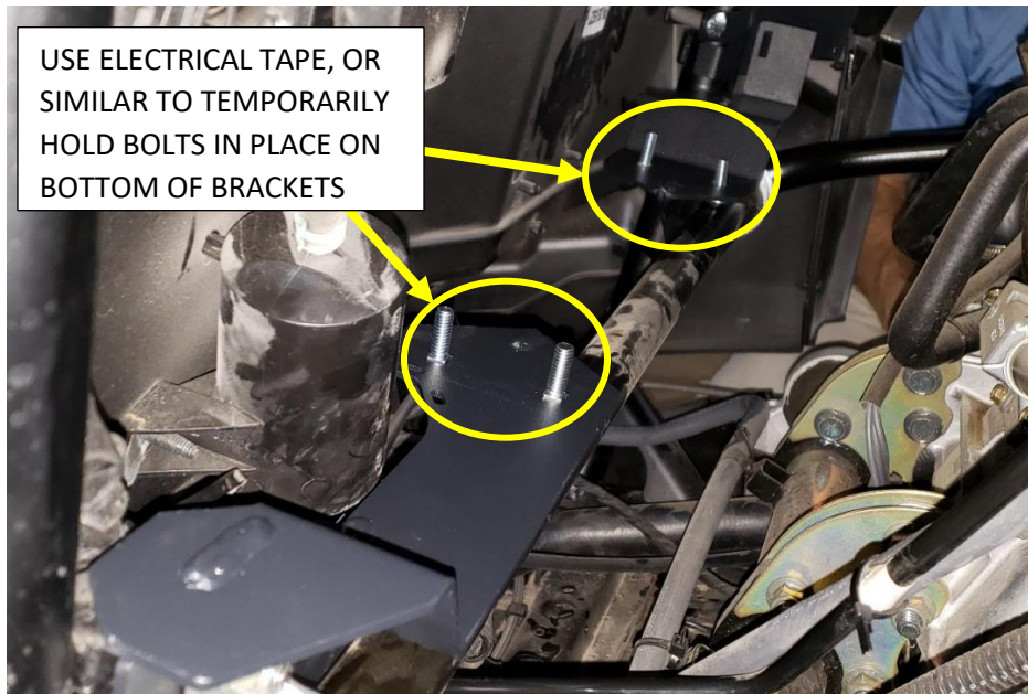
Figure 11 - Air Tank Brackets with Air Tank Bolts taped to bottom
