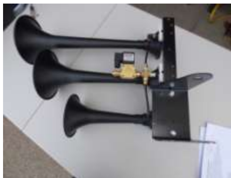
Solenoid and fitting installed
