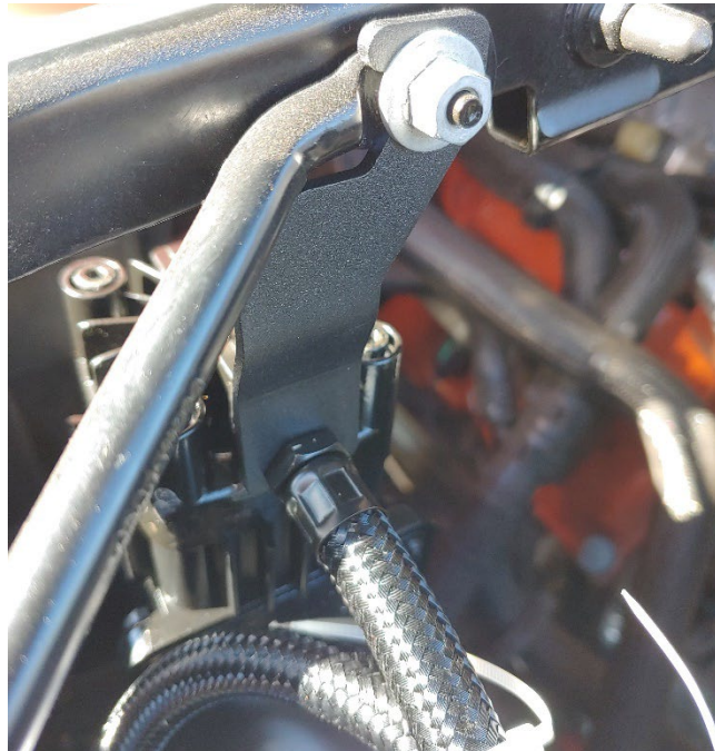
Figure 21- Anchor Bracket, Installed
