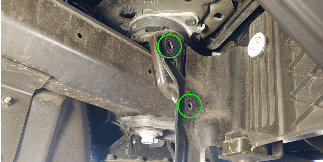
Figure 28- OEM Bolts, Removed
