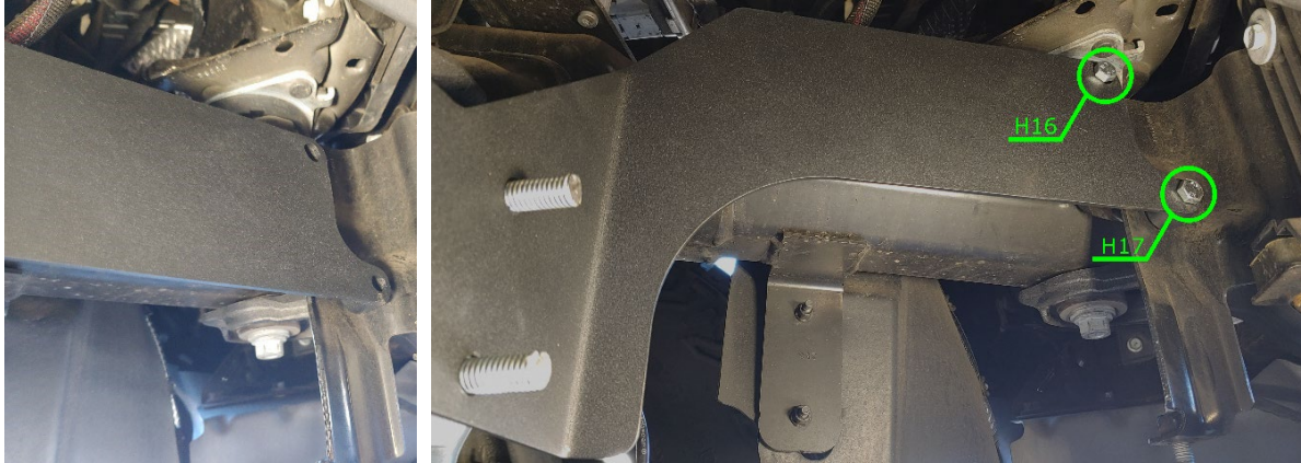
Figure 30- Primary Tank Bracket Installation 2, Step 11
