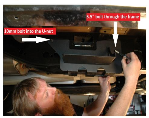
The 5.5 inch bolt will have a flat washer for each side. Lift the bracket so that the bolt. with one flat washer, can pass through the frame, use the supplied flat washer, lock washer, and bolt on the inside of the frame rail.
