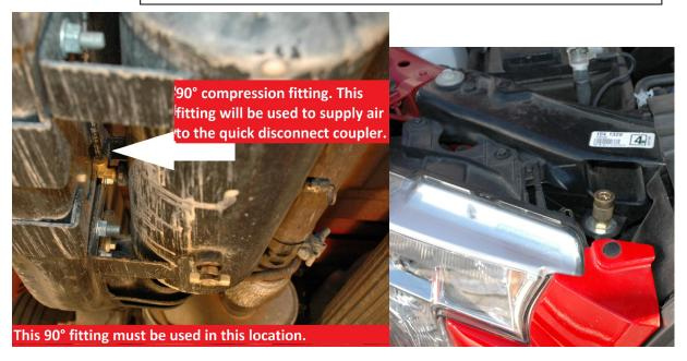
The airline to feed the quick connect coupler, will be installed on the port between the mounting legs, it should be positioned to have the airline running in the direction of the location you will mount the quick connect coupler. Install the airline, and tighten the compression fitting, before mounting the tank to the bracket. The coupler can be mounted using the supplied bracket, or custom mounted, such as through the bumper.
