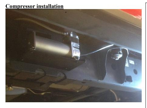
Once the bracket is securely in its final mounting position, the compressor can be mounted to the shelf. The compressor should be mounted as shown. facing forward, this will allow for easy routing of the stainless steel braided leader hose over the frame, and ultimately plumbed into the tank. The ground for the compressor can be attached to a paint free metal surface of the vehicle, and the red 12v+ wire can be wired to the relay (pin 87)
