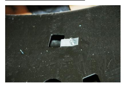
The Extruded U-nut will be installed by sliding it through the square hole, so that the threaded nut will be positioned behind the circular opening.
