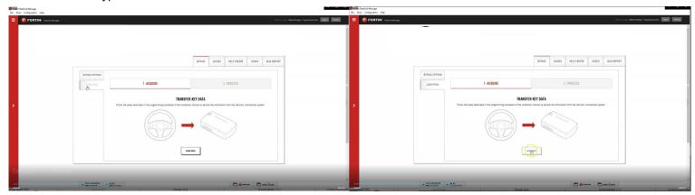
4. Wait while the updater reads data from the remote starter. Once it is done it will update the remote starter and you will need to wait again. You will see a status bar at the bottom of the screen. When it gets to 100%, the Dcryptor process is complete.
