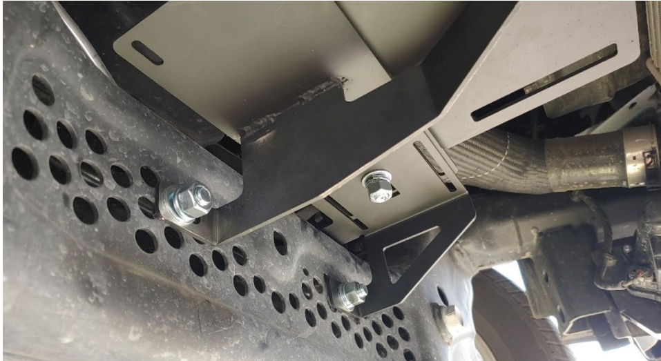
Figure 11- Tank / Compressor Bracket Installation 3
