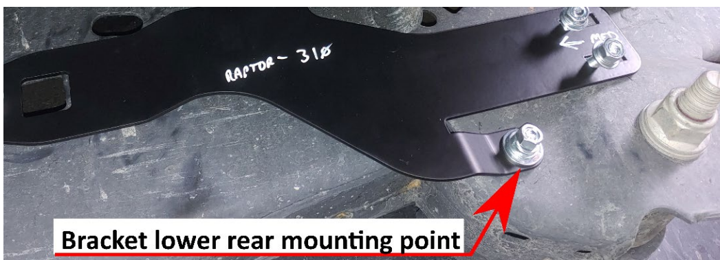
Figure 30- RAPTOR-310 Lower Mounting Point Installed
