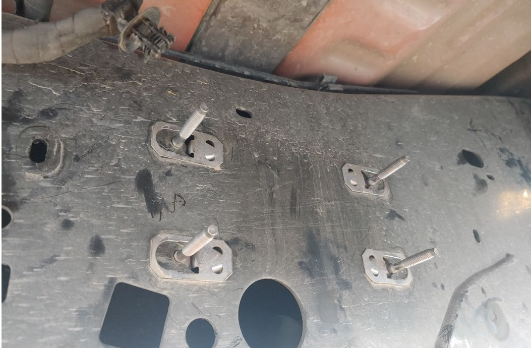
Figure 33- Module & Wire Harness Removed
