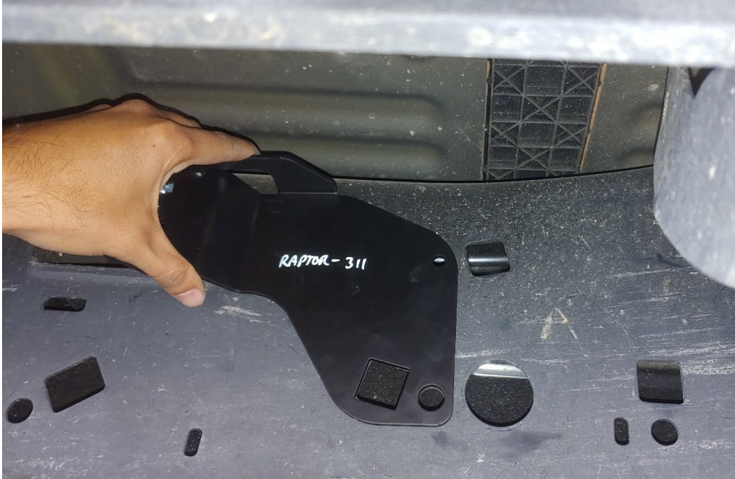
Figure 24- Installation Orientation of the Front Horn Bracket
