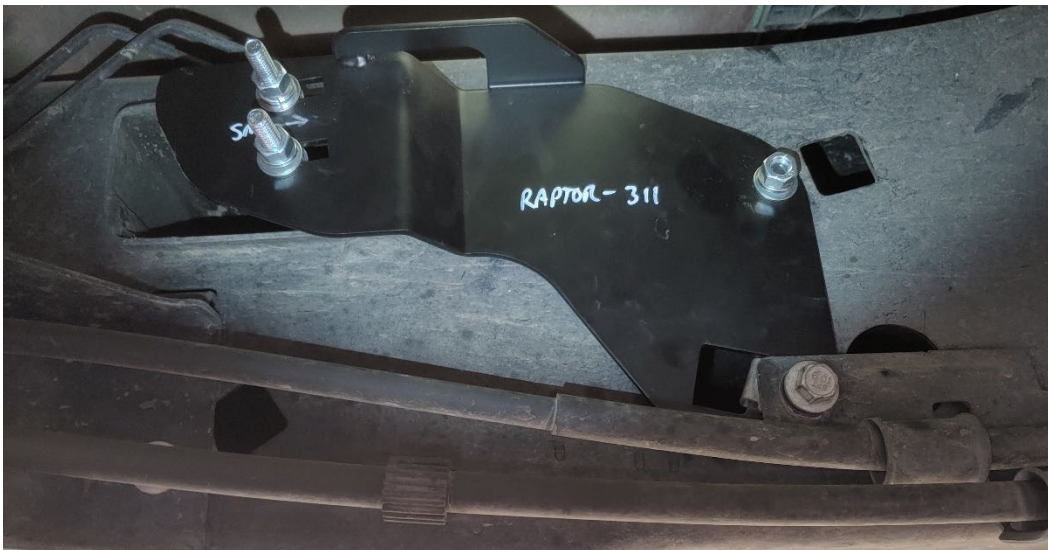
Figure 27- Front Horn Bracket Installed
