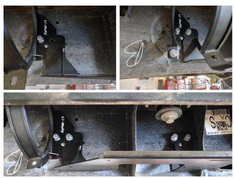
Figure 9- Compressor & Front Tank Bracket Installed
