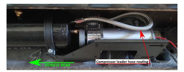
Figure 17- Air Tank Installation 3
