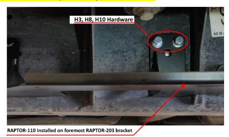
Figure 8- Compressor Bracket, One Side Installed
