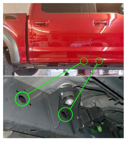
Figure 6- Nut Plates (RAPTOR-203) Install Locations
