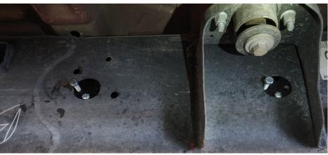
Figure 7- Nut Plates (RAPTOR-203) Installed
