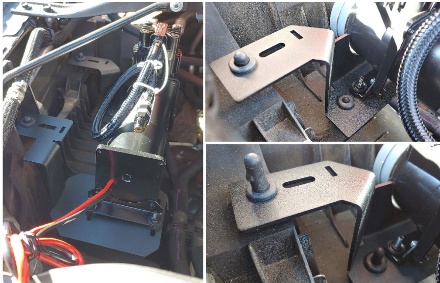
Figure 17- Compressor Bracket, Installed
