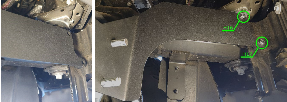
Figure 30- Primary Tank Bracket Installation 2, Step 11
