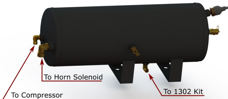
Figure 42- Final Plumbing of Air System
