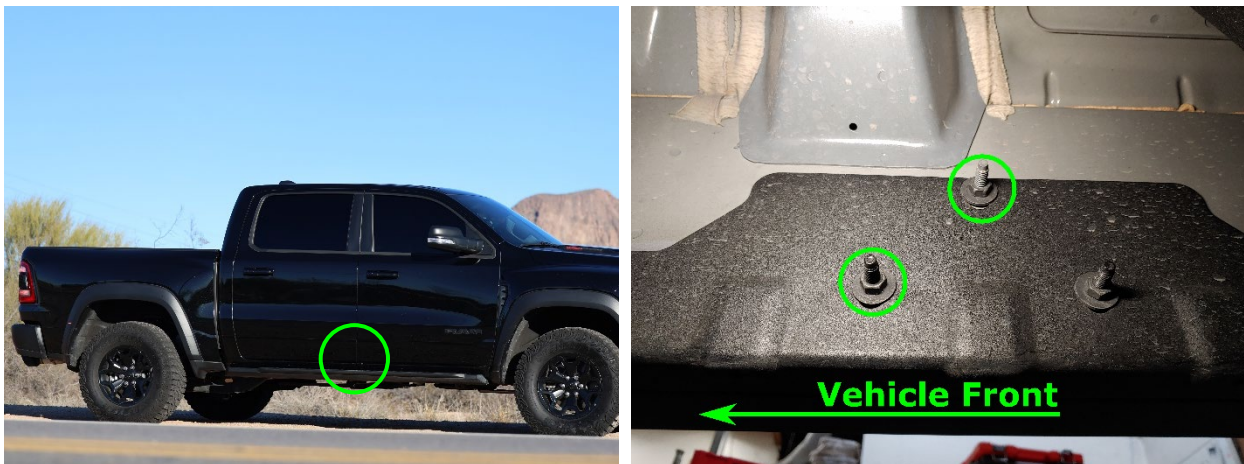
Figure 40- Medium Horn Bracket, Location & Mounting Spot
