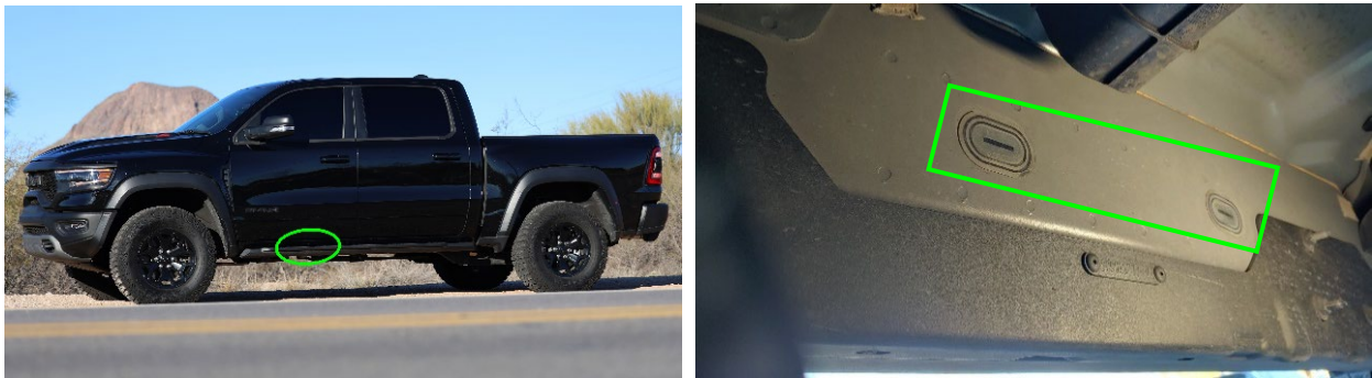
Figure 32- Mounting Location of Ore Brackets
