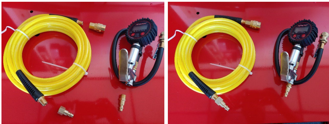
Figure 9- Accessory Fittings Installation
