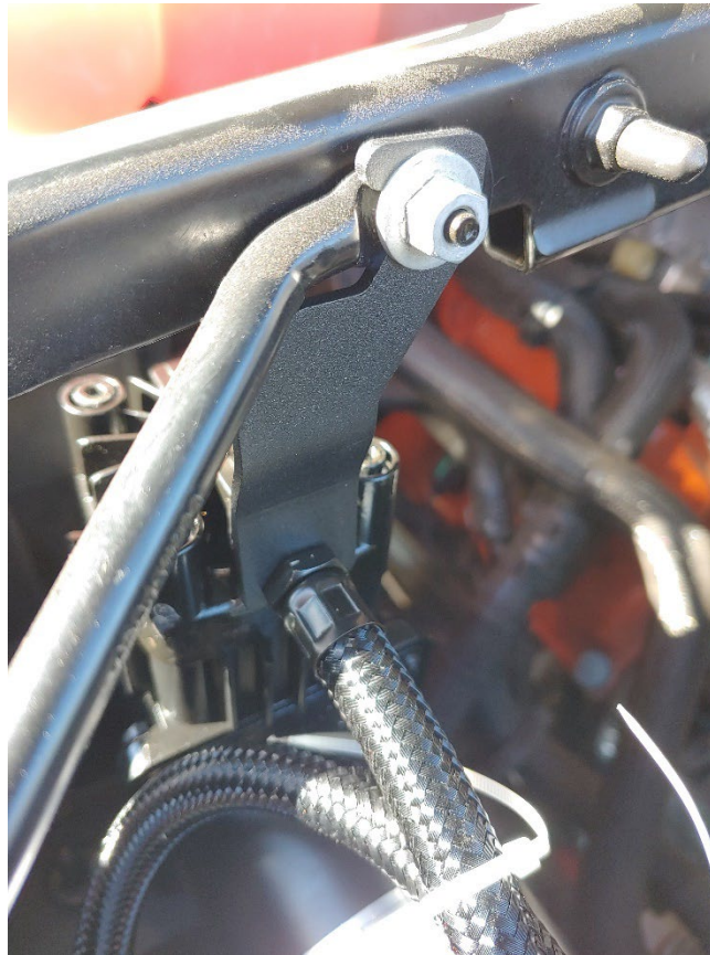
Figure 21- Anchor Bracket, Installed
