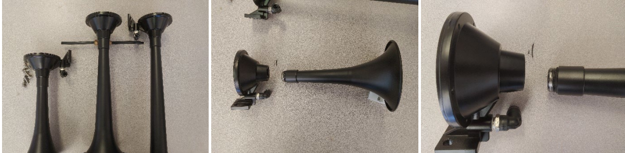
Figure 10- Air Horn Separation
