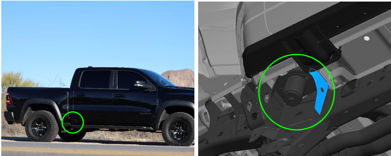
Figure 37- Small Horn Bracket, Location & Mounting Spot
