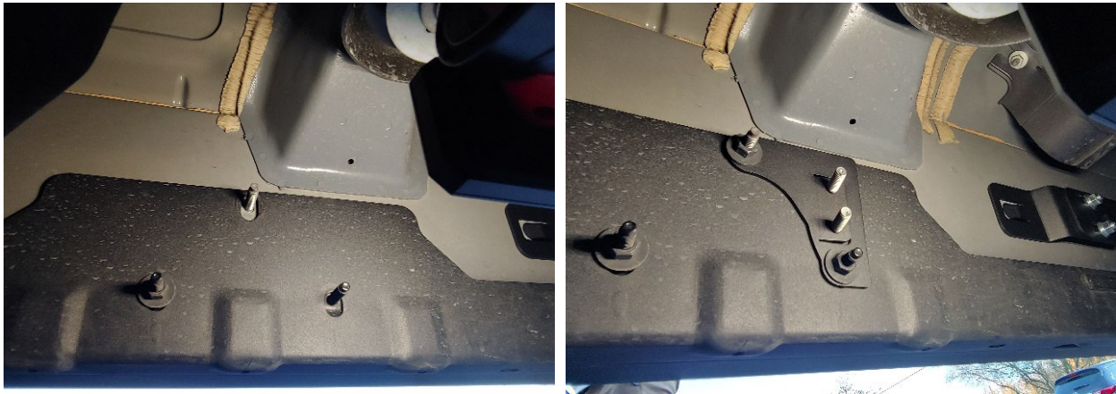
Figure 35- Driver Horn Bracket, Installed
